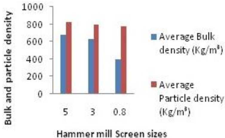
Figure 6. Bulk and particle density of grinded palm kernel shell.
