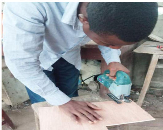
Plate 6. Cutting the plywood with electric jigsaw. Author's fieldwork (2019).
