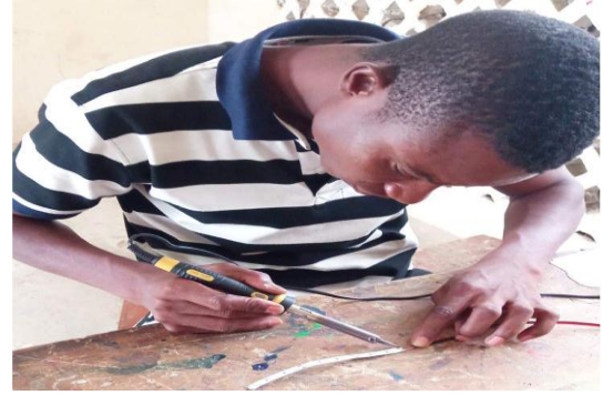
Plate 8. Soldering the LED strip to the wire. Author's fieldwork (2019).
