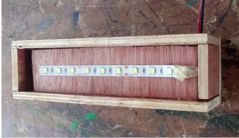
Plate 11. The LED strip being layed into the base casement. Author's fieldwork (2019).
