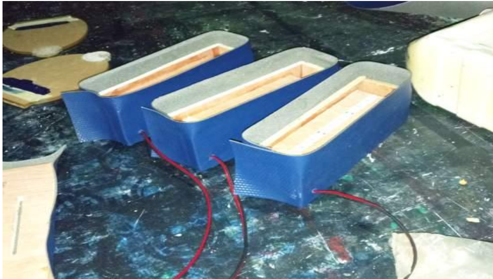
Plate 12. Wrapping lamp casing with leather. Author's fieldwork (2019).
