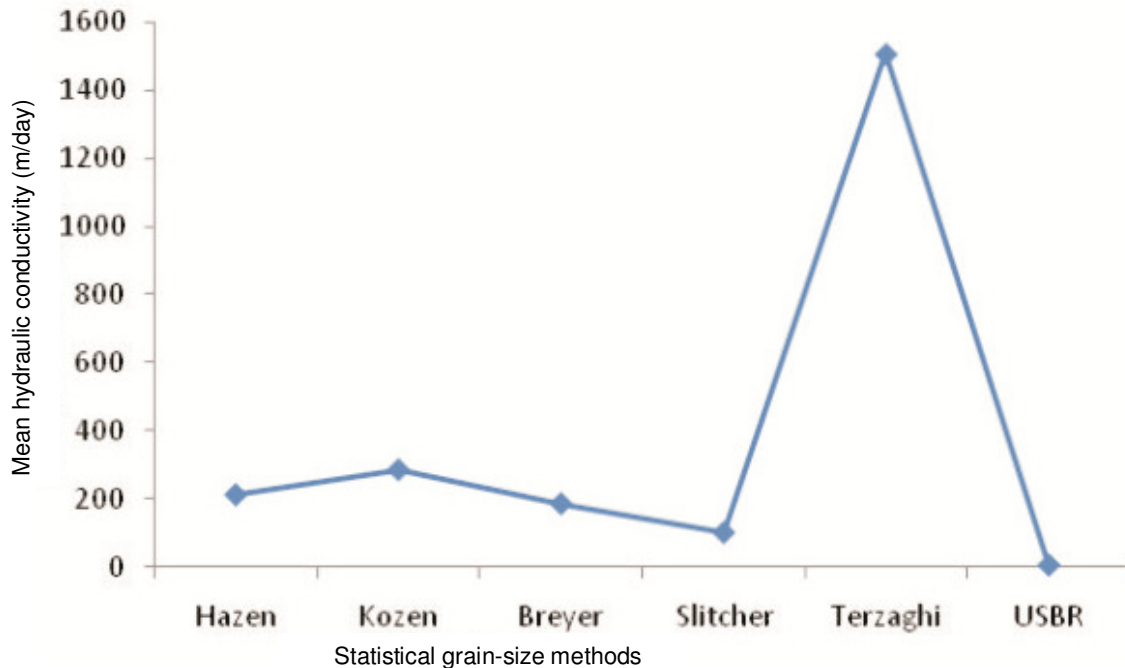
Figure 4. Plots of hydraulic conductivity versus grain-size methods.
