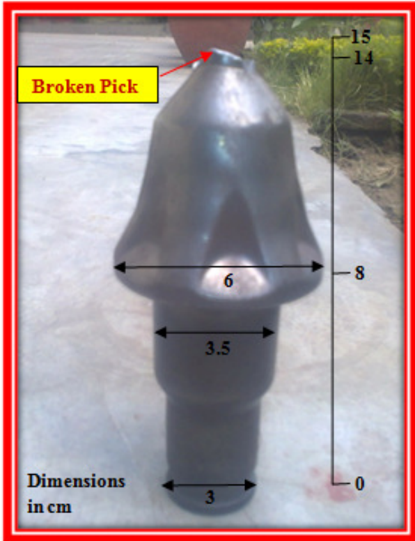
Figure 3. Broken pick due to overload.
