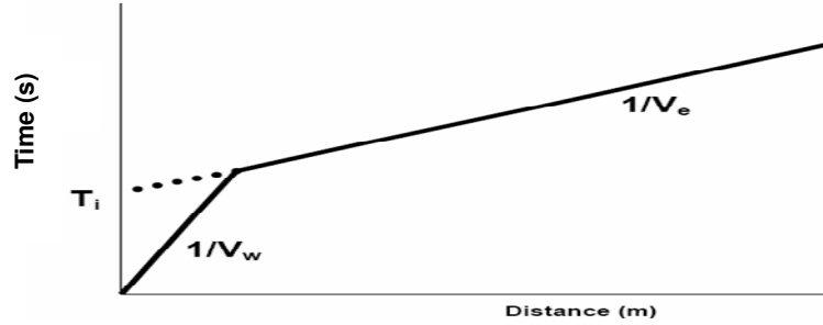
Figure 4. T-X plot for a 2-layer case.
