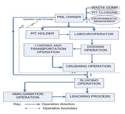
Figure 4. ASM conceptual model of operation.
