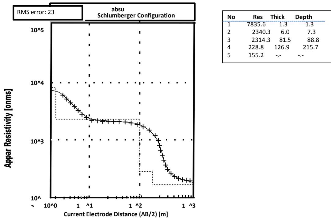
Figure 4. Result of computer modelled curve for VERS A<sup>10</sup>.
