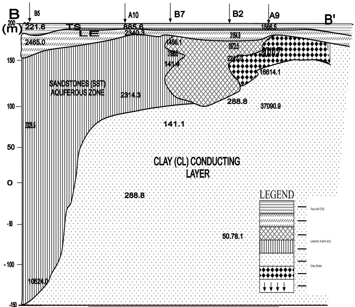
Figure 6. Geoelectrical section along BB'.
