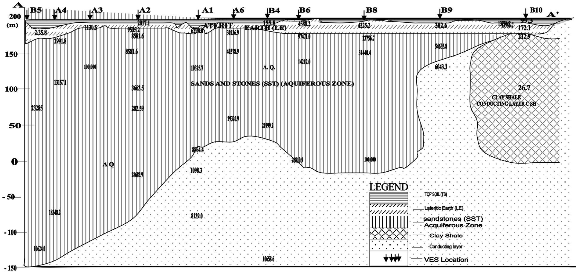
Figure 5. Geoelectrical section along AA'.
