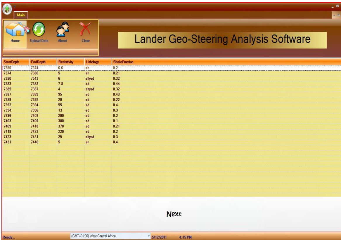
Figure 5. Offset well resistivity tool response data.
