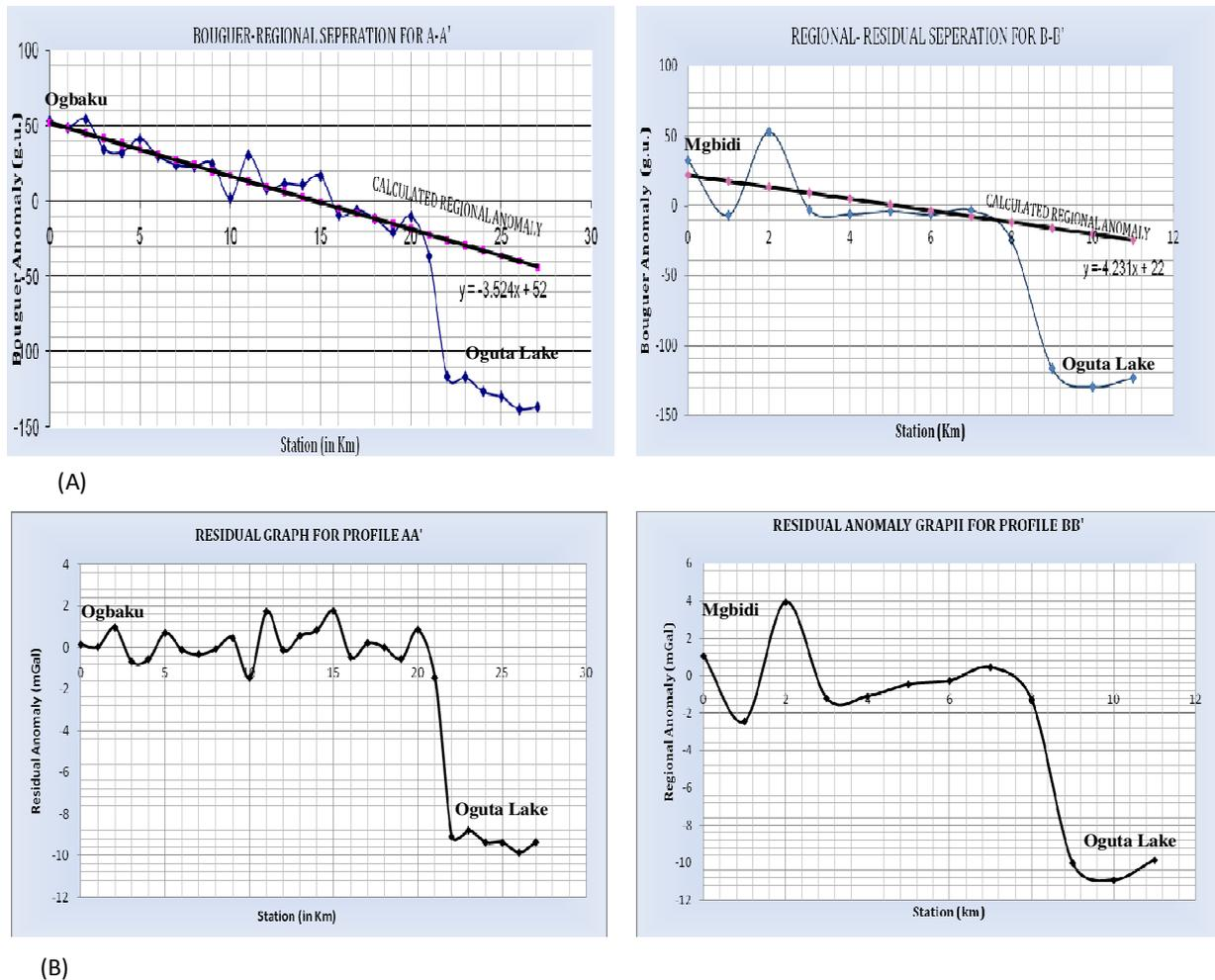
Figure 5. (a) Regional – residual separation graphs for profiles A-A' and B-B', (b) Residual anomalies for Profiles A-A' and B-B'.
