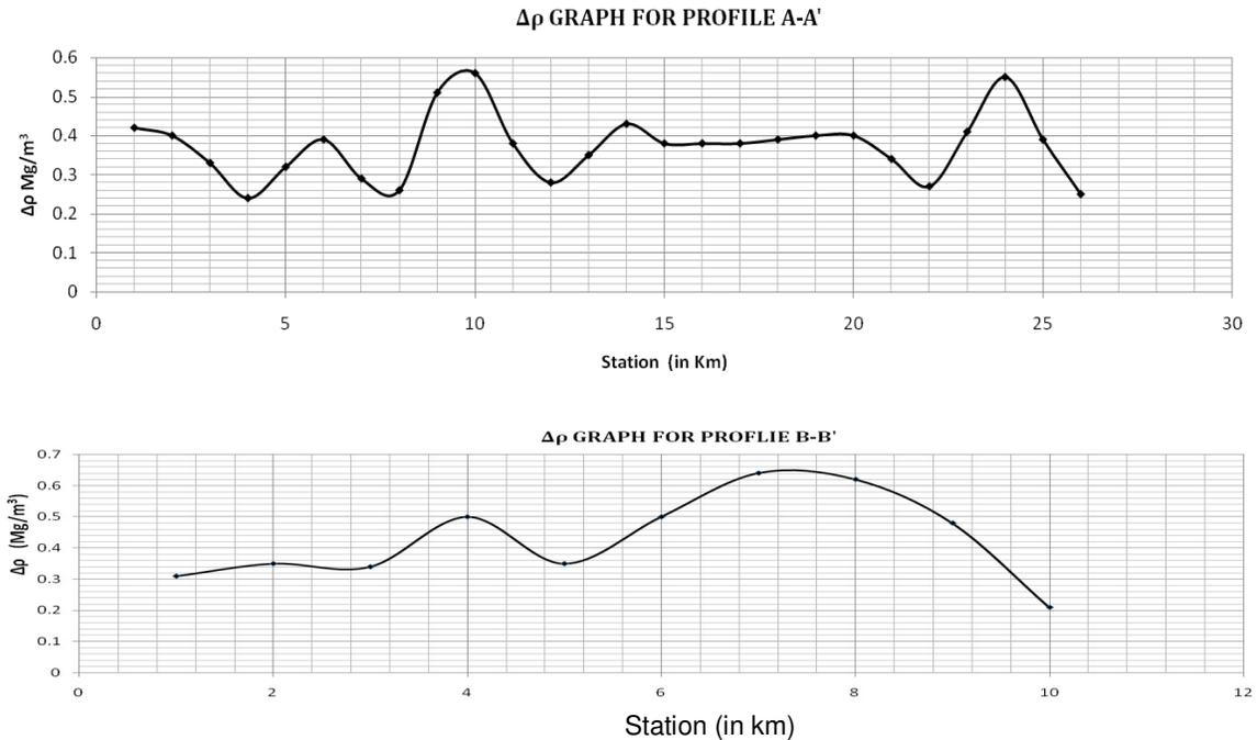
Figure 4. Density contrast graph for Profiles A-A' and B-B'.
