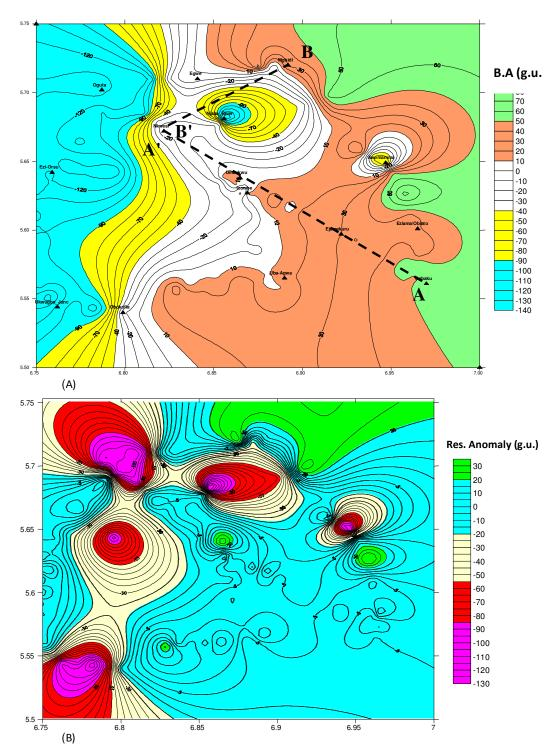
**Figure 6.** (a) The Bouguer anomaly map of the study area showing the two profiles of major interest A-A' and B-B', (b) Residual contour map of the area.
