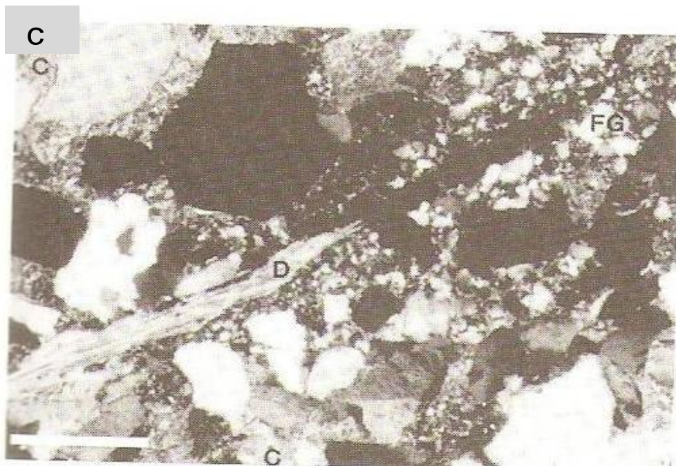
Figure 5c. Microfault, with associated fracture gouge (FG) and partially infilled by Dawsonite.
