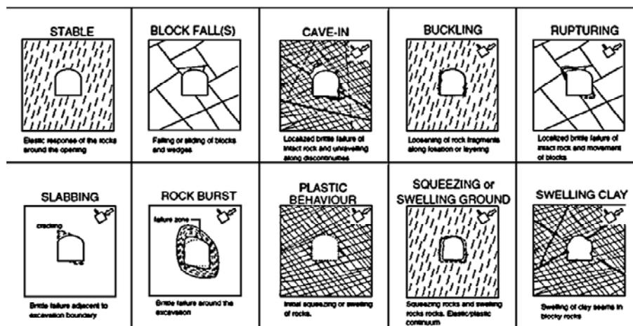
**Figure 3.** Some types of behavior types in underground openings (partly from Martin et al., 1999; Hoek et al., 1995).
