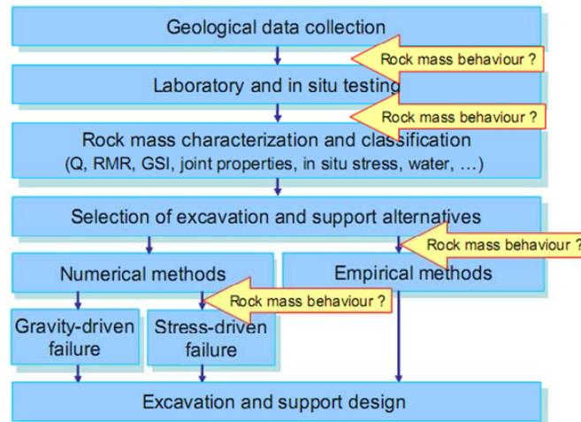
**Figure 2.** Site characterization approach for standard geotechnical projects; the arrows are where a sound understanding of rock mass behavior is needed (Kaiser et al., 2000).
