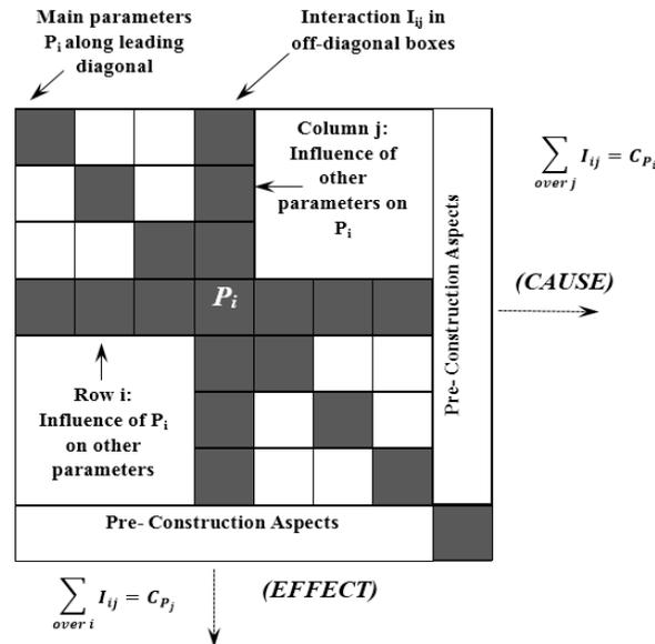
**Figure 5.** Summation of coding values in the row and column through each parameter to establish the cause and effect co-ordinates (modified from Hudson, 1992).
