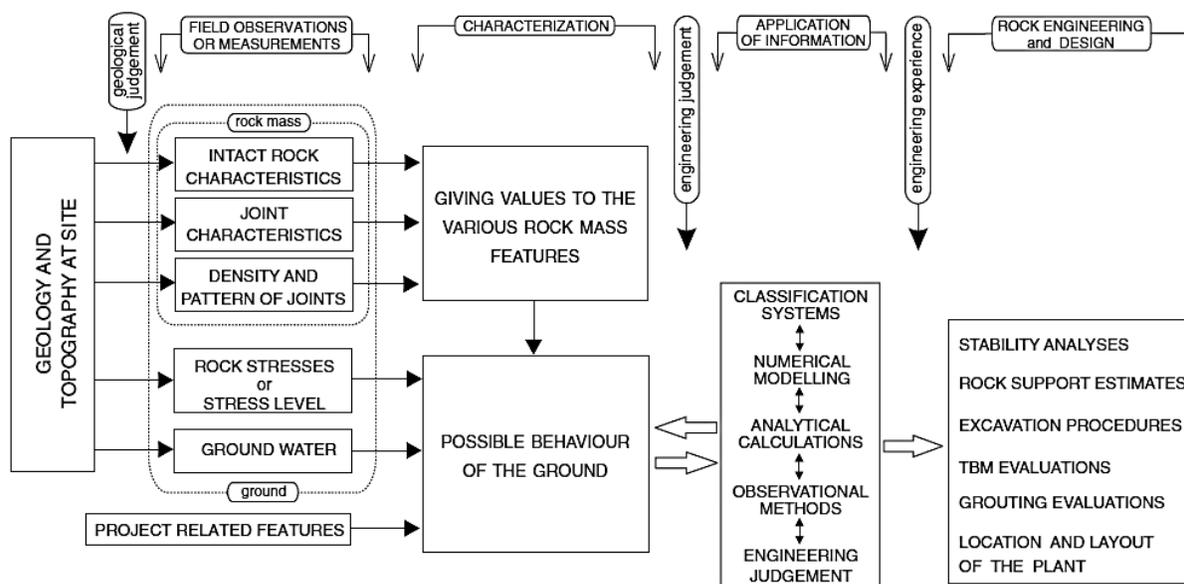
**Figure 1.** The principle relationships between ground behavior and rock engineering and design (Taken from / reproduced from Stille and Palmstrom, 2003).
