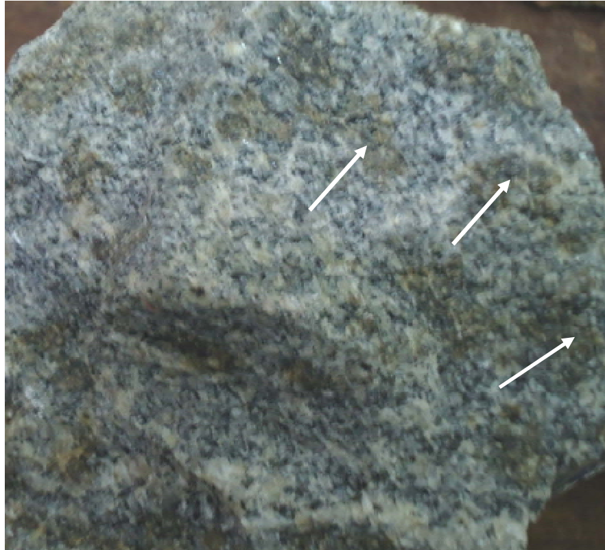
Figure 3. Hand specimen of early gneiss with charnockitic spots. Arrows indicate the charnockitic spots.
