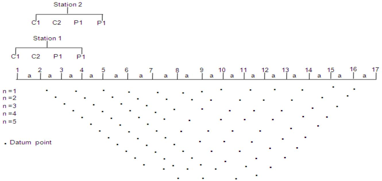
**Figure 6.** Sequence measurement used to build up pseudo section for the ERT data in the study area.
