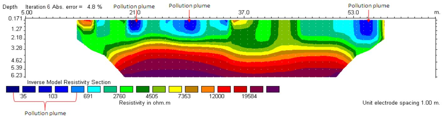
Figure 12. ERT result for traverse 3 acquired in Ebhokhuala 100m away from the dumpsite.
