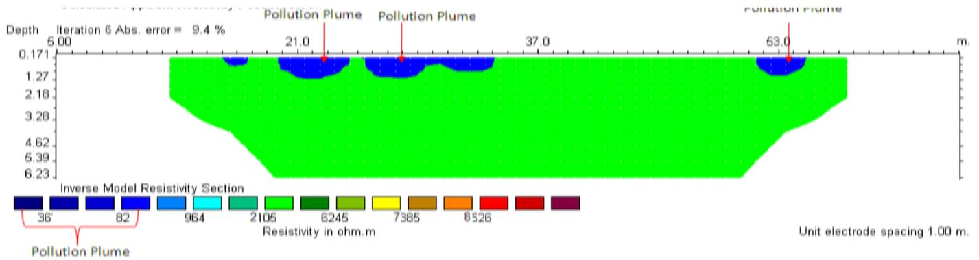
Figure 11. ERT result for traverse 2 acquired in Ebhokhuala 50m away from the dumpsite.
