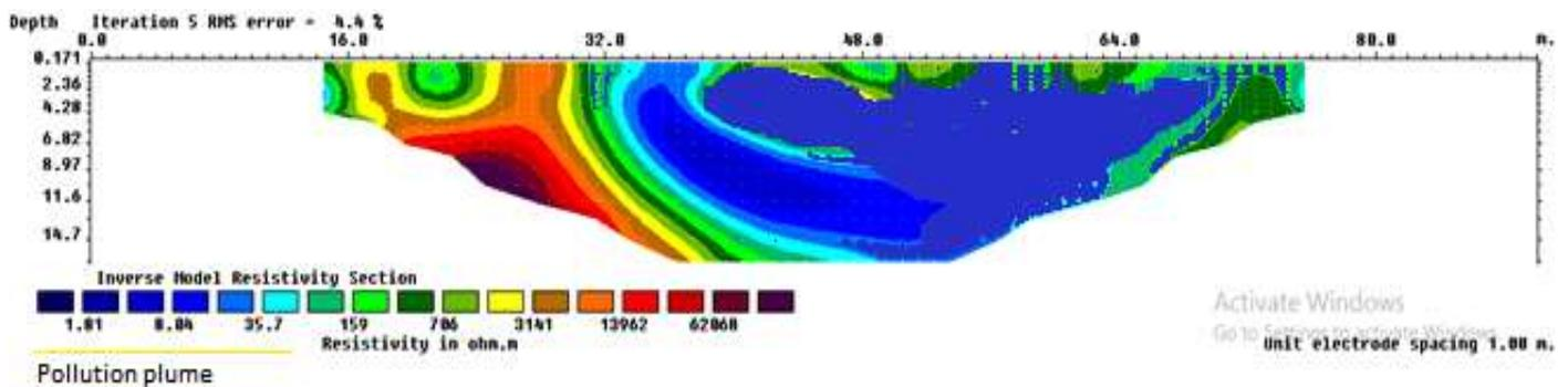
Figure 14. ERT result for traverse 2 acquired in Agbede 50m away from the dumpsite.
