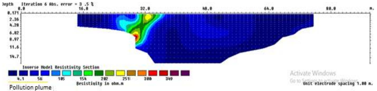
Figure 13. ERT result for traverse acquired in Agbede 2m away from the dumpsite.
