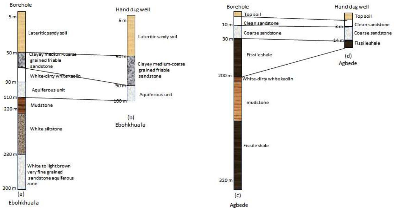
Figure 8. Correlation of hand dug wells with borehole in Ebokhuala and Agbede, Edo State.
