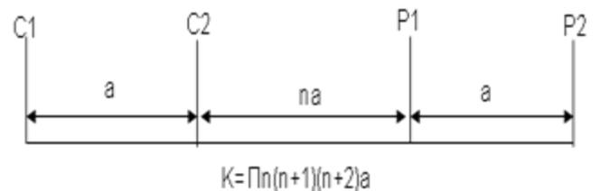
**Figure 5.** Dipole-Dipole electrode array.
