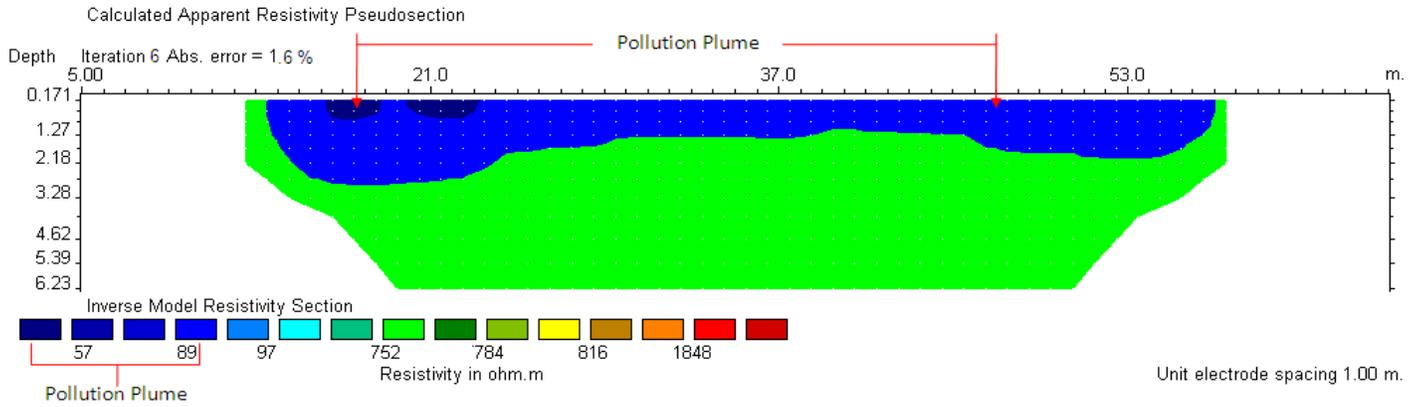
Figure 10. ERT result for traverse 1 acquired in Ebhokhuala 2m away from the dumpsite.
