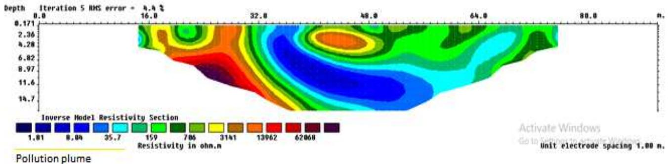
Figure 15. ERT result for traverse 3 acquired in Agbede 100m away from the dumpsite.
