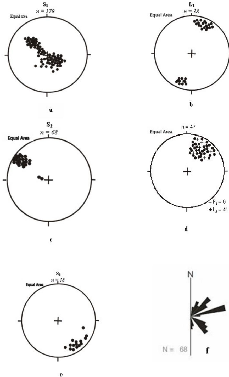
**Figure 7.** Equal-area Schmidt lower hemisphere projection of structural data: (a): Poles to  $S_1$  foliations; (b)  $L_1$  mineral and stretching lineation; (c) Poles to  $S_2$  foliations; (d)  $L_2$  Stretching lineation and  $F_2$  fold axes; (e) Poles to  $S_3$  foliation and (f): Rose diagram of fracture planes depicting three main structural trends (N30-N40E, N70-N80E and N140-N150E).
