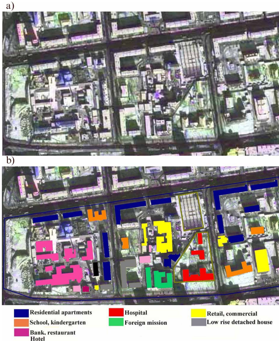
Figure 2. The images created by Brovey transform (a) and the related interpretation (b).
