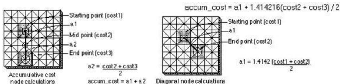
**Figure 2.** Accumulative cost calculation.
