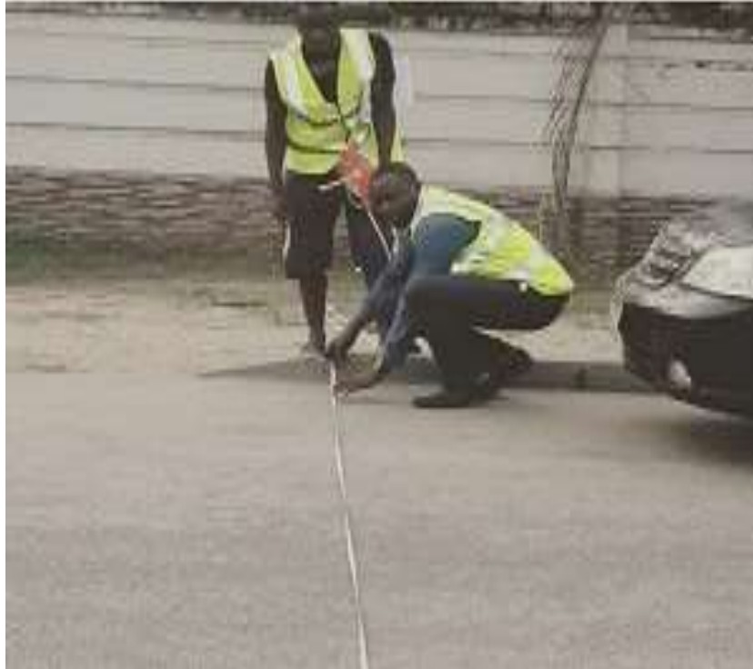
Figure 3. Picture illustrating how the width of roads under study was measured.
