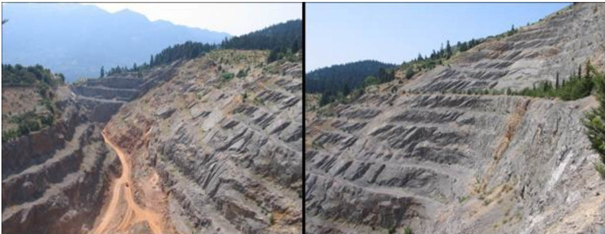
Figures 8. (a) Koukouvista 5, opencast mine. (b) Distinguish vertical mining fronts (Mertzanis et al., 2004a).
