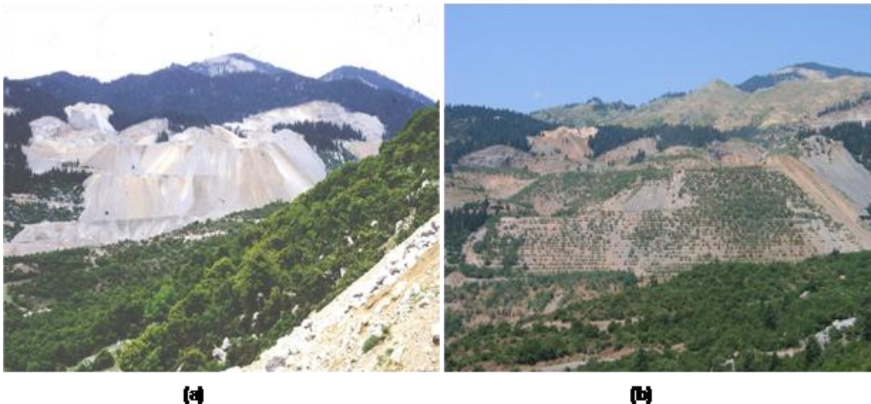
Figures 12. (a) Inert materials deposits (bauxite mining spoils) on Koukouvista 5 opencast mine, before restoration (Mertzanis et al., 2006). (b) Inert materials deposits, on Koukouvista 5 opencast mine, at an early stage of restoration (Mertzanis et al., 2004a).
