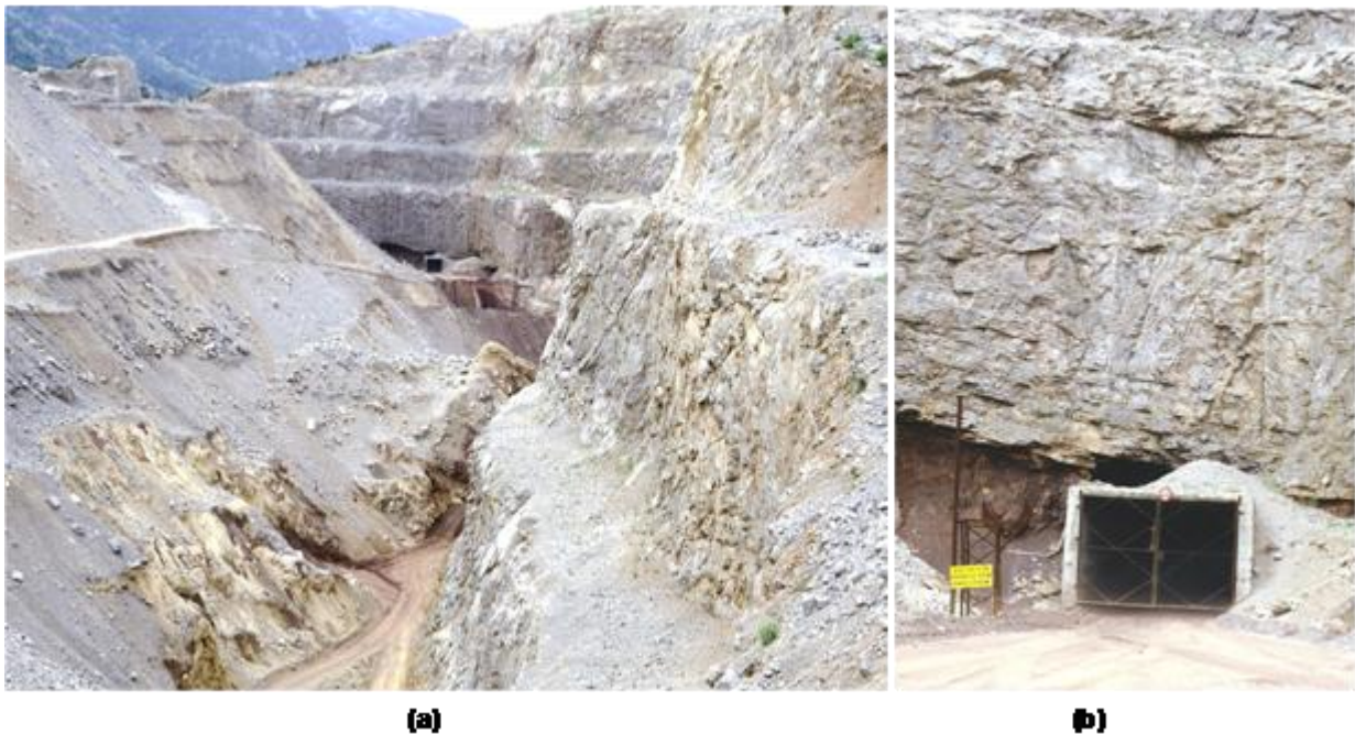
Figures 7. (a) Combination of “open cast” and “underground” mining methods, in the study area. (b) Detail of the tunnel entrance (Mertzanis et al., 2006).
