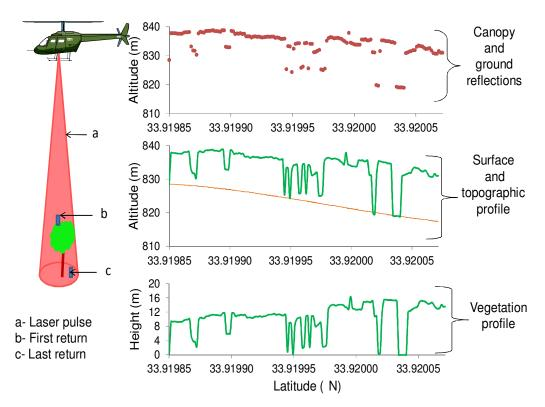
**Figure 1.** Illustration of airborne laser profiling and processing of vegetation profile; Main components in Portable Airborne Laser Systems fitted in aircraft include Infrared Laser Altimeter (ILA), Video Tape Recorder (VTR) and Differential GPS.
