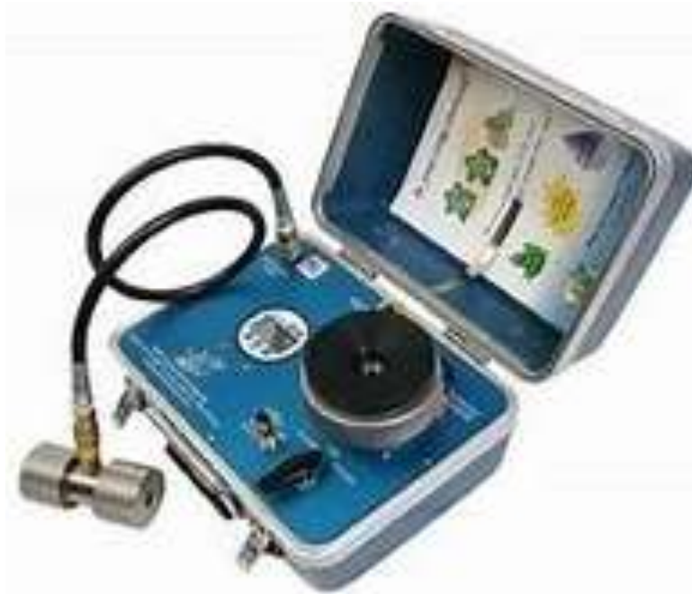
Figure 1. Pressure chamber for measuring stem and leaf water potential. Source: https://edaphic.com.au/plant-and-leaf-water-potential/water-potential-pressure-chamber-standard/
