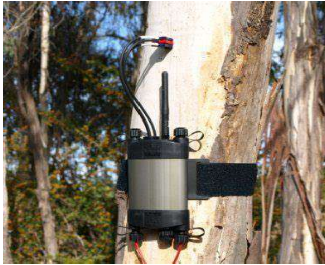
Figure 3. SFM1 Sap flow meter to measure transpiration or sap flow in plants.
