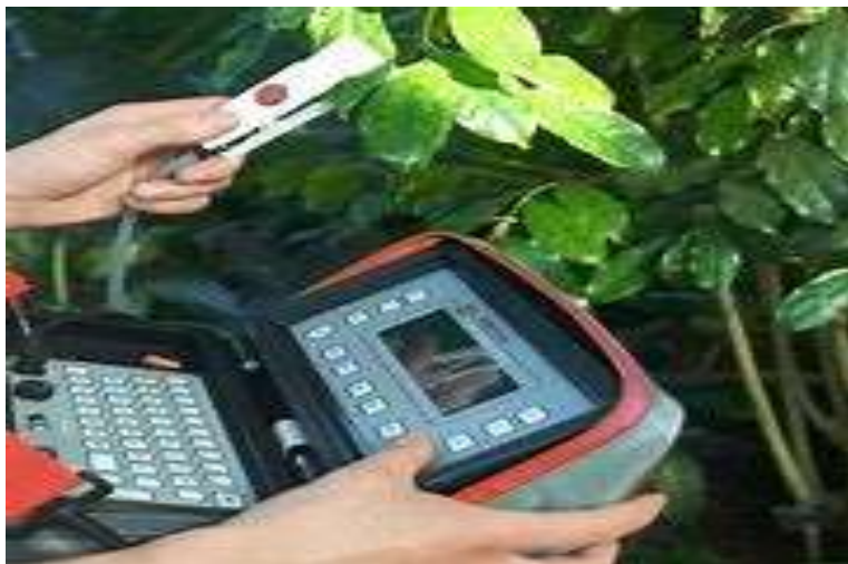
Figure 2. Porometer for measuring leaf stomatal conductance. Source: www.delta-t.co.uk
