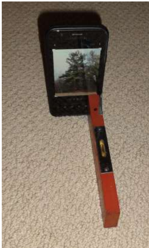
Figure 1. The instrument used in the Photo Method: a cell phone taped to a small level.
