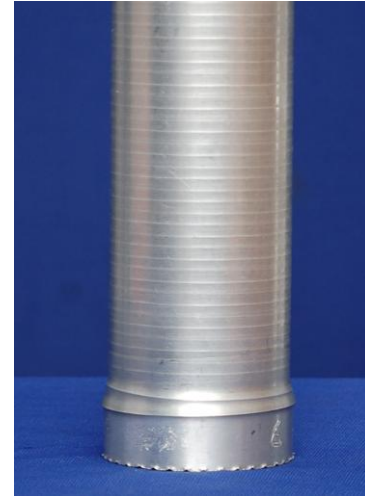
Figure 5. A flow formed tube with scratch marks on the surface.
