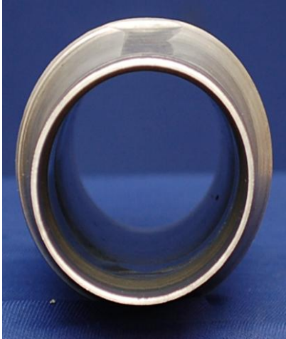
Figure 7. A flow formed tube with large ovality problem.
