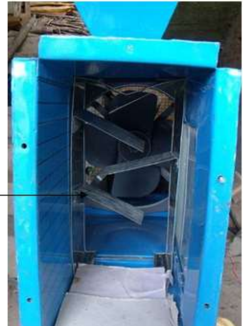
Figure 14. Vertical cascade fitted in the screening chamber.
