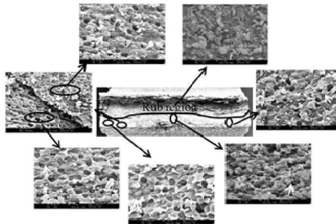
**Figure 6.** Map of overall crack propagation direction.
