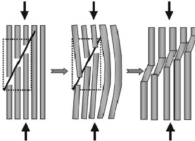
**Figure 7.** Schematic model of the damage zone leading to kink band formation (Source: Garland et al., 2001 used with permission).
