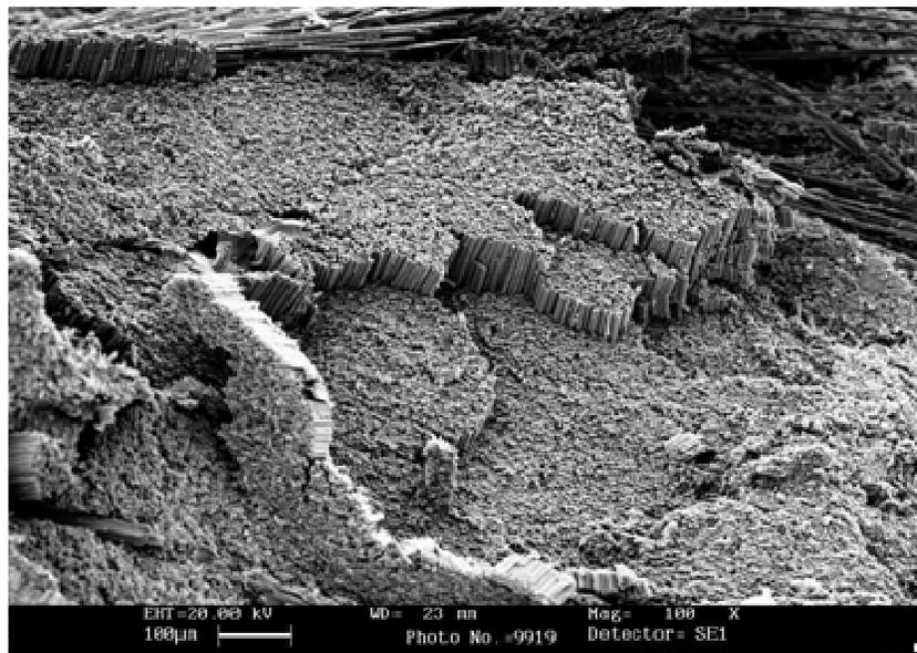
**Figure 5a.** Stepped fibre fracture.
