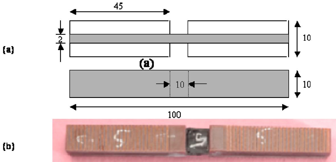
Figure 1. (a) Schematic representation and (b) Actual photograph of the compression specimen.
