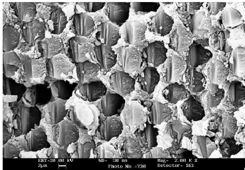
**Figure 5d.** Chop marks typical of failure under compressive load.
