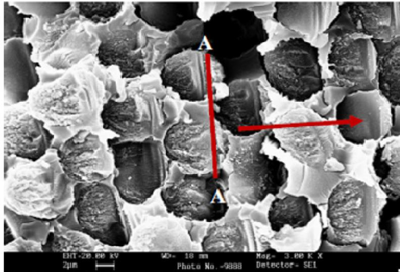
**Figure 5f.** Local crack propagation direction indicated by an arrow perpendicular to neutral axis AA.
