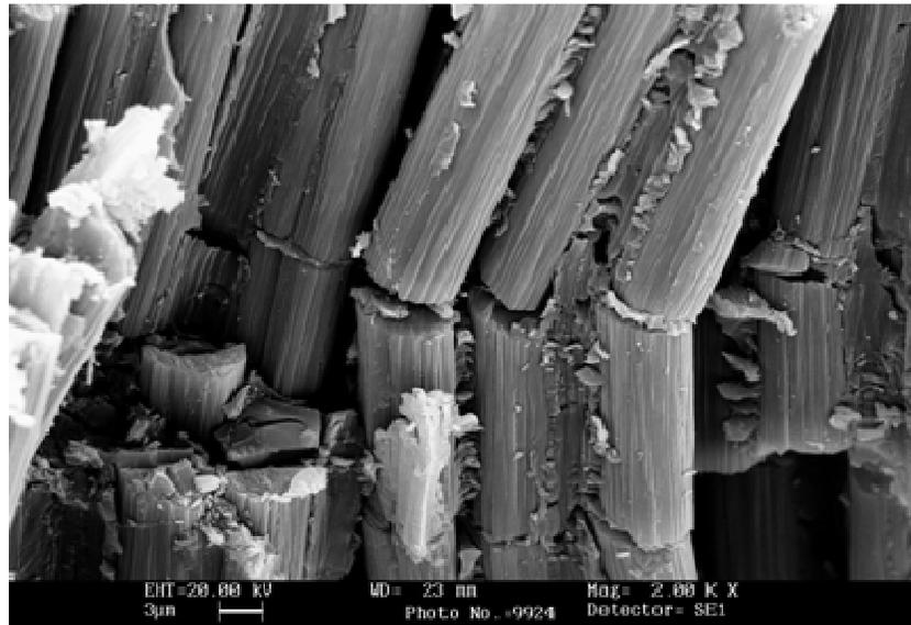
**Figure 5c.** Microbuckling/Kinking.
