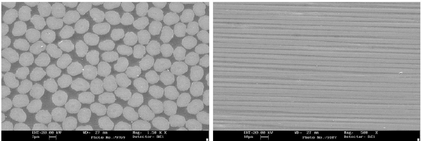
Figure 2. SEM micrograph showing (a) longitudinal and (b) cross sectional uniform distribution of carbon fibers in epoxy matrix.
