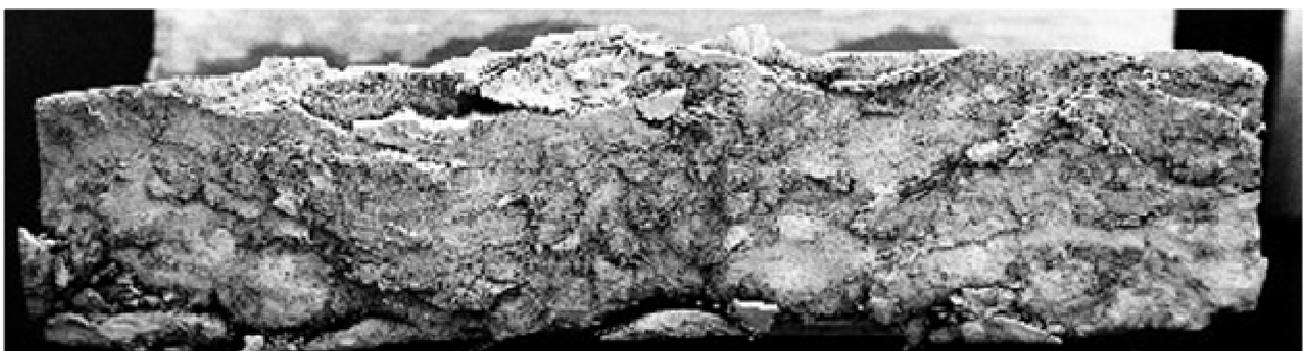
Figure 3. Fracture surface of compression failed test coupon.
