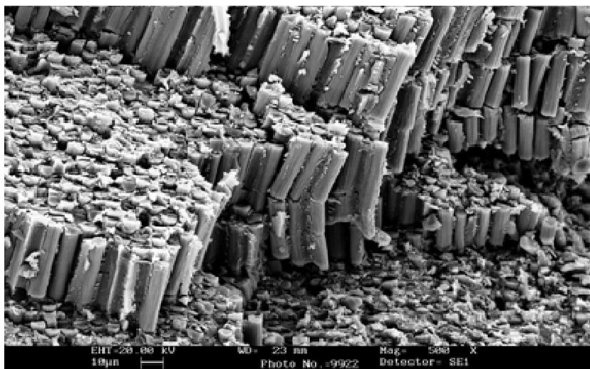
**Figure 5b.** Fibre fracture by micro buckling and fracture at different heights.
