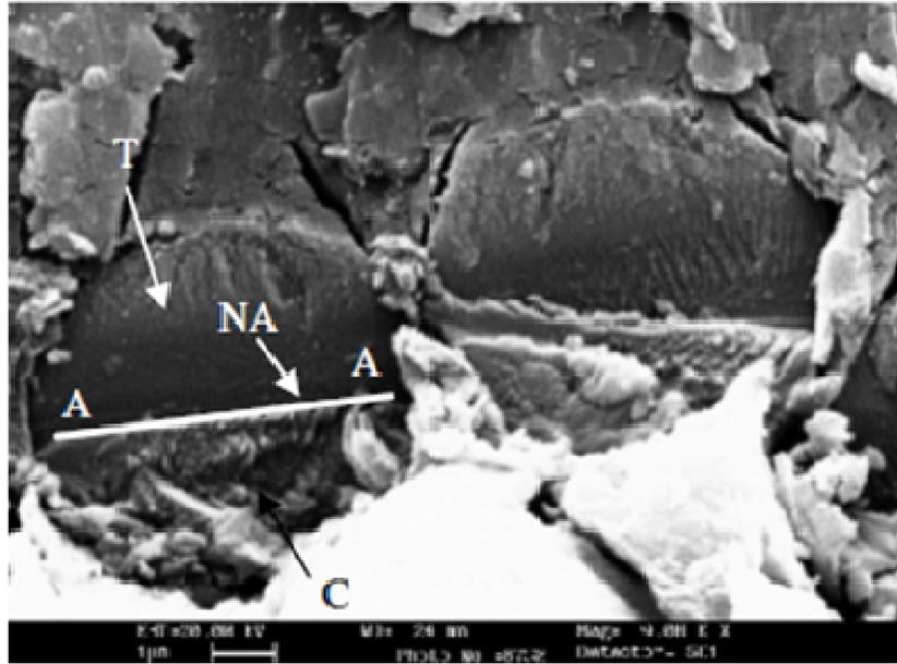
**Figure 5e.** High magnification fractograph showing chop marks separating tension and compression by neutral axis.
