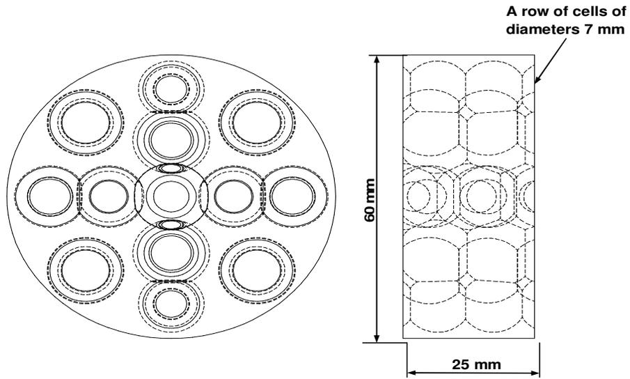
Figure 1. A generic multiple orifice physical scale model designed using a CAD package.
