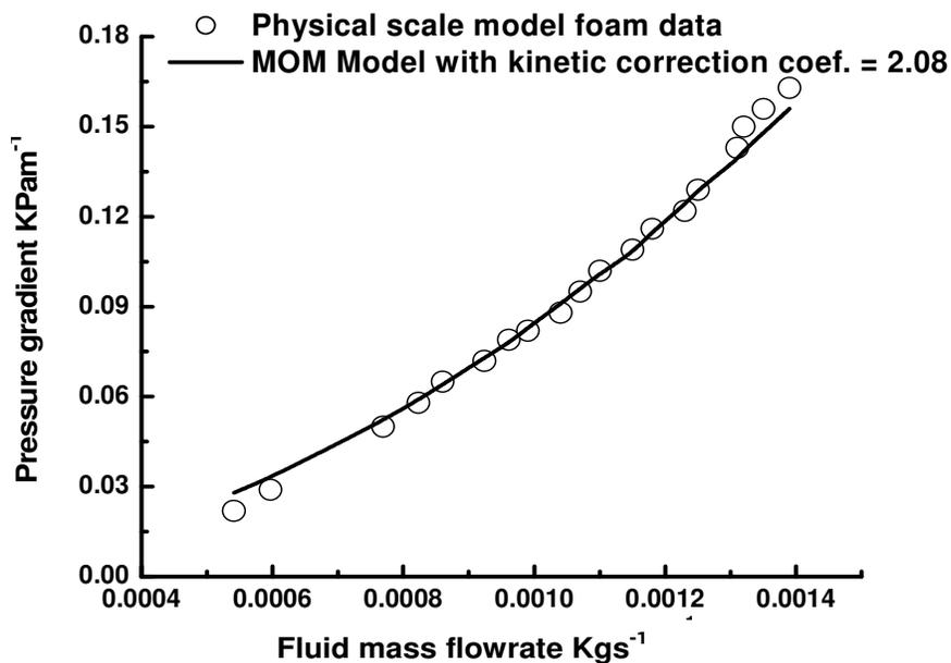
**Figure 5.** Graph of pressure gradient vs. fluid flow rate in a physical scale model foam sample, for the calibration of the MOM model. Reynolds number is from 35 to 99.
