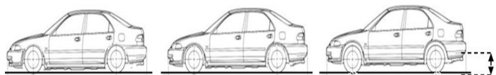
Figure 34. Shorter distance between the center of gravity (car body) and ground in high speed results in more stability.
