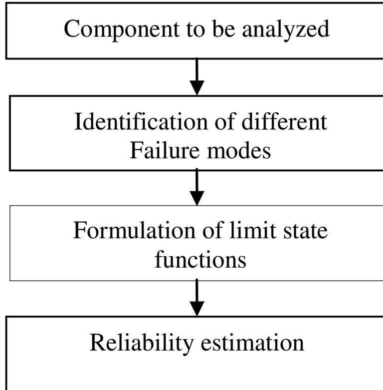
**Figure 3.** Flow chart representing the steps involved in performing the reliability analysis.
