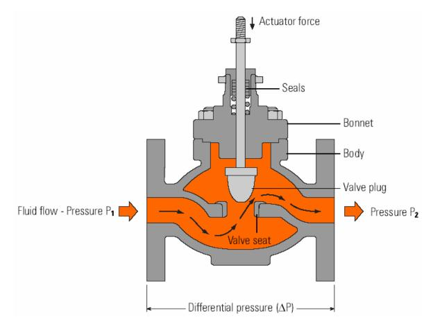
Figure 1. Flow through a single seat two-port globe valve SC-GCM-58 (2005).
