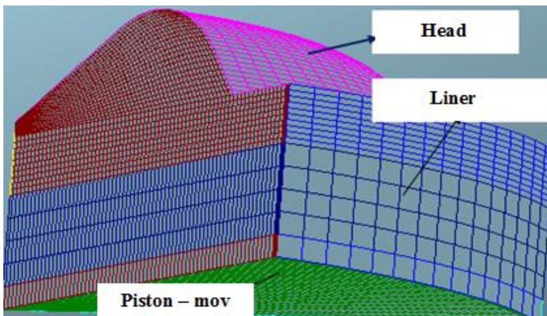
**Figure 2.** Boundary condition that used in simulation.
