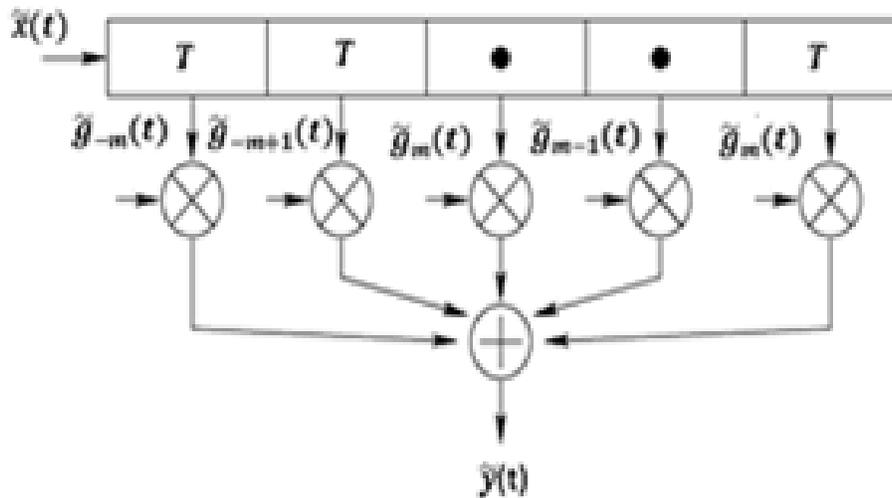
Figure 2. Uniformly spaced TDL model for a discrete multipath channel.
