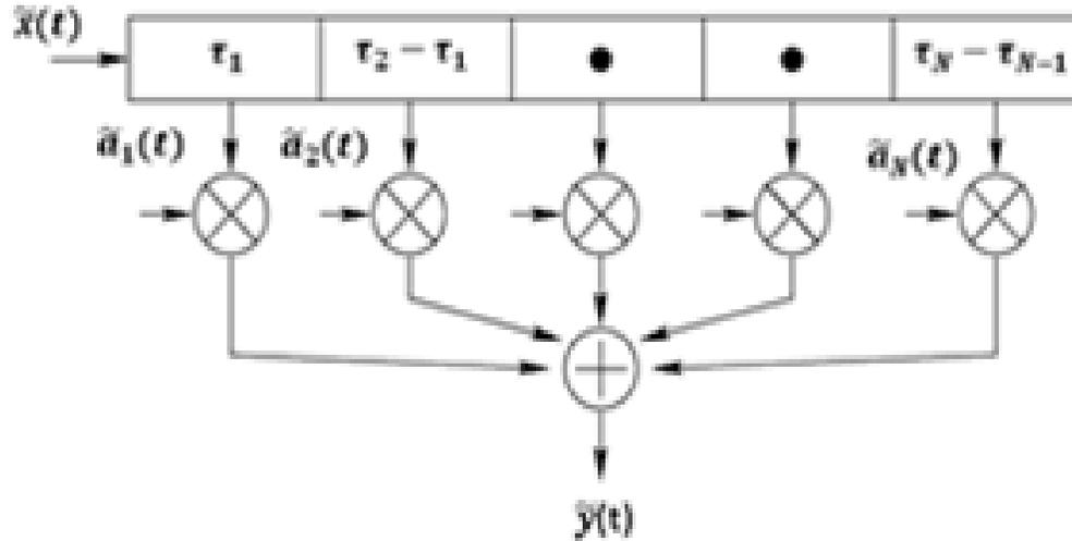
Figure 1. A variable delay TDL model for discrete multipath channels.
