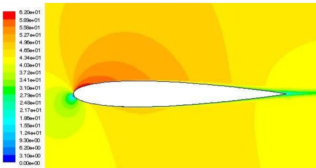
**Figure 10.** Contours of velocity magnitude at 3° angle of attack with the Spalart-Allmaras turbulence model.
