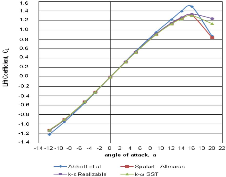
**Figure 4.** Comparison between experimental data from Abbott et al and three different turbulent models simulation results of the lift coefficient curve for NACA 0012 airfoil.
