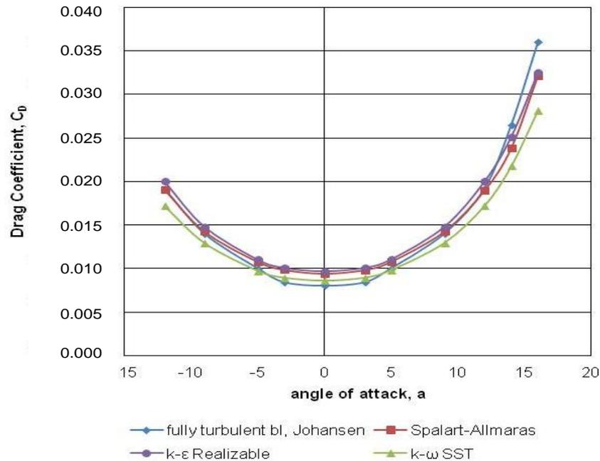
**Figure 6.** Comparison between experimental data for fully turbulent boundary layer from Johansen and three different turbulent models simulation results of the drag coefficient curve for NACA 0012 airfoil.
