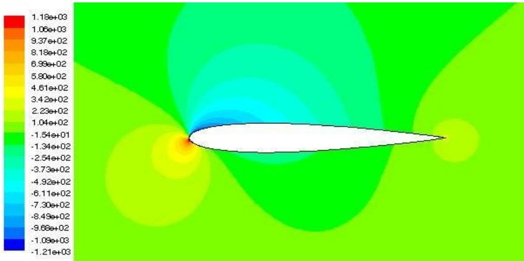
**Figure 8.** Contours of static pressure at 3° angle of attack with the Spalart – Allmaras turbulence model.
