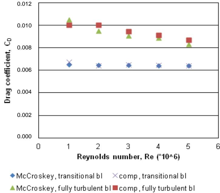
**Figure 7.** Comparison between experimental data for fully turbulent and transitional boundary layer from McCroskey and simulation results with the split grid of the drag coefficient curve for NACA 0012 airfoil at zero angle of attack and at various Reynolds numbers.
