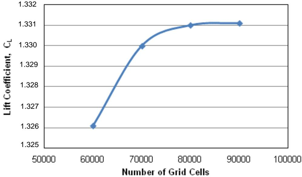
Figure 1. Curve of lift coefficient at stall angle of attack against number of grid cells.
