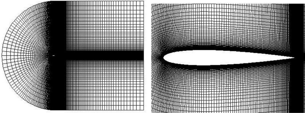
Figure 2. Mesh around NACA 0012 airfoil (left) and detail close to the airfoil (right).
