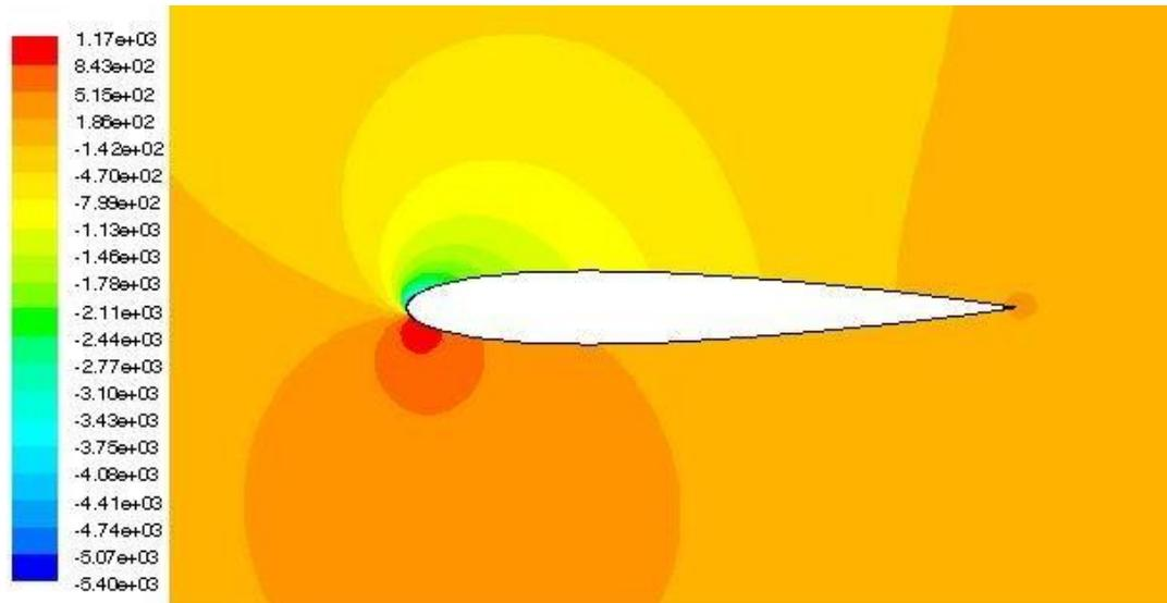
**Figure 9.** Contours of static pressure at 9° angle of attack with the Spalart – Allmaras turbulence model.
