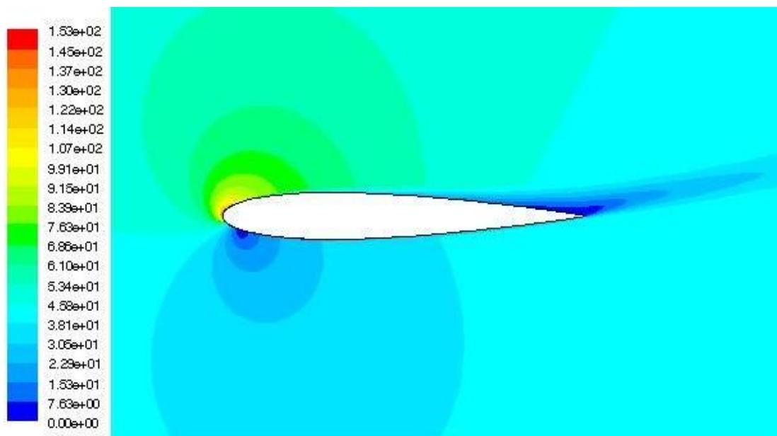
Figure 12. Contours of velocity magnitude at 16° angle of attack with the Spalart-Allmaras turbulence model.
