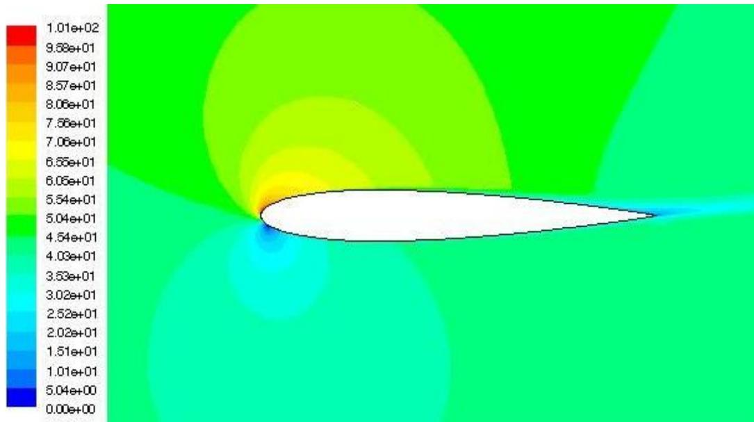
Figure 11. Contours of velocity magnitude at 9° angle of attack with the Spalart-Allmaras turbulence model.
