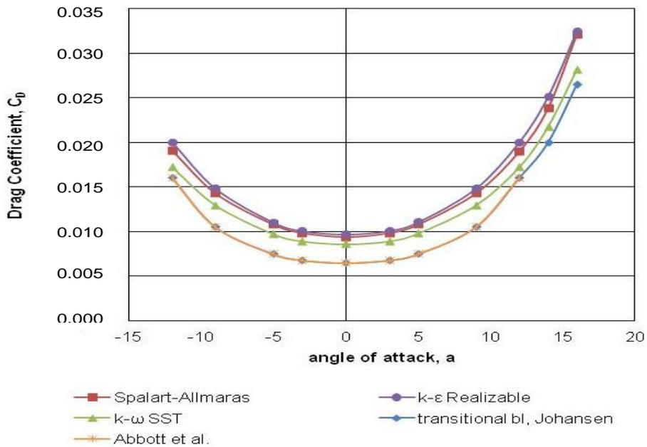
**Figure 5.** Comparison between experimental data from Abbott and Von Doenhoff (1959) and Johansen (1997) for transitional boundary layer and three different turbulent models simulation results of the drag coefficient curve for NACA 0012 airfoil.
