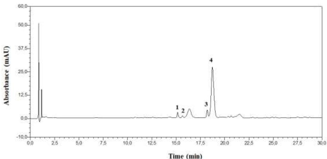
**Figure 1.** HPLC fingerprint chromatogram ( $\lambda=337$  nm) of ELPA. Mobile phase: ACN (B): 0.2% (w/w) formic acid (A) (0-30 min, 5-20% of B). Flow rate: 0.6 ml/min. Injection volume: 0.6  $\mu$ L. Column temperature: 30°C. Peaks: 1 - isoorientin; 2 - orientin; 3 - vitexin; 4 - isovitexin.
