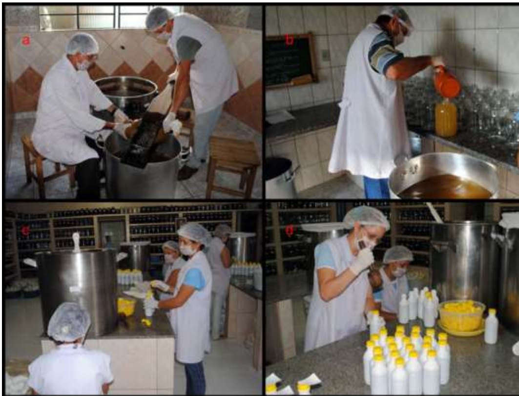
Figure 6. Pressing for sludge separation (a); storage of simple formulation (b); formulation of compounds (c and d) in the production process of herbal medicines in the GEP. Source: Records of the GEP.
