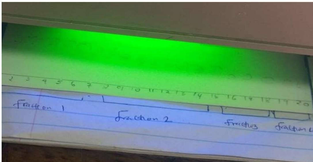
**Figure 1.** TLC chromatogram showing four fractions obtained from column chromatography of the dichloromethane extract.
