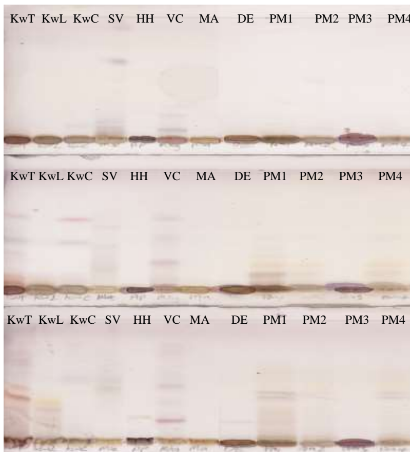
Figure 2. Chromatograms of plant decoctions showing various coloured compounds that reacted with vanillin-sulphuric acid reagent. Different colours developed after heating the sprayed chromatograms at 110°C. Kw (T, L, C): K. wilmsii (twigs, leaves, corm); SV: S. viminalis ; HH: H. hemerocallidea ; VC: V. capensis ; MA: M. angustifolia ; DE: D. elata ; PM (1, 2, 3, 4): Different Tšhikwana powders.
