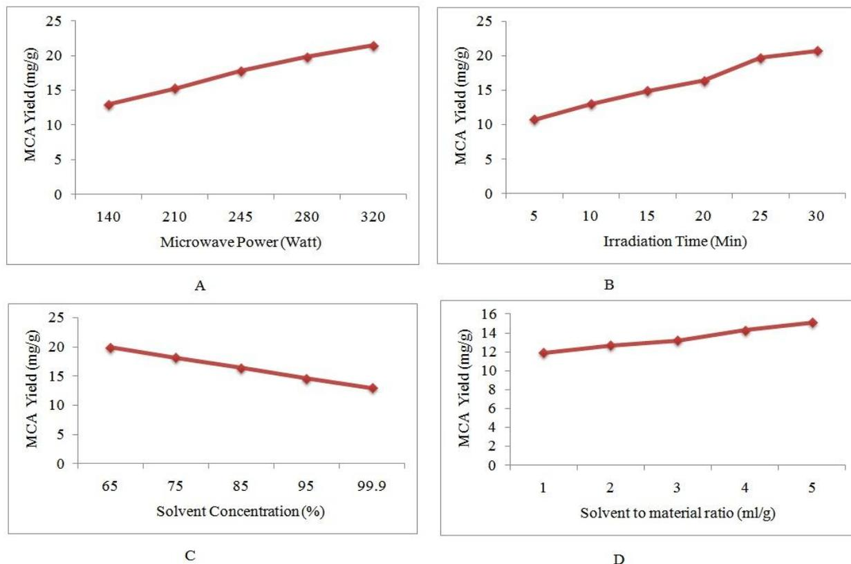
**Figure 1.** Effect of different factors on MCA yield. (A) Microwave power (95% ethanol, solvent ratio 10 ml/g, 78°C, 10 min, two cycles); (B) Duration of irradiation (140 W, 95% ethanol, solvent ratio 10 ml/g, 78°C, two cycles); (C) Solvent concentration (140W, solvent ratio 10 ml/g, 78°C, 10 min, two cycles); (D) solvent to material ratio (140 W, 95% ethanol, 78°C, 10 min, two cycles).
