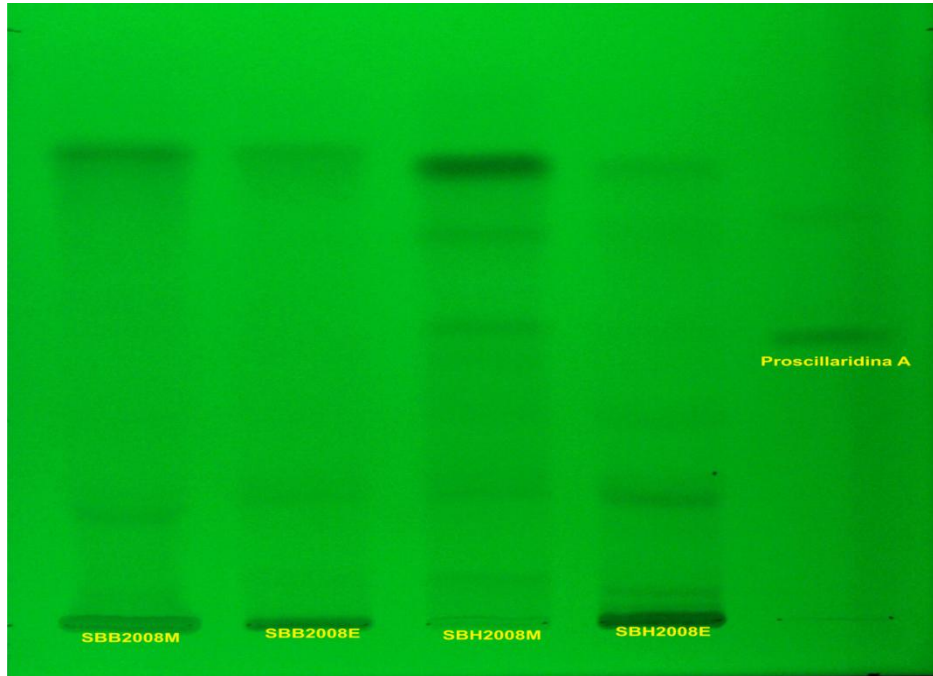
Figure 3. The chromatogram of the extracts of Scilla bifolia harvested in 2009 at UV 254 nm.
