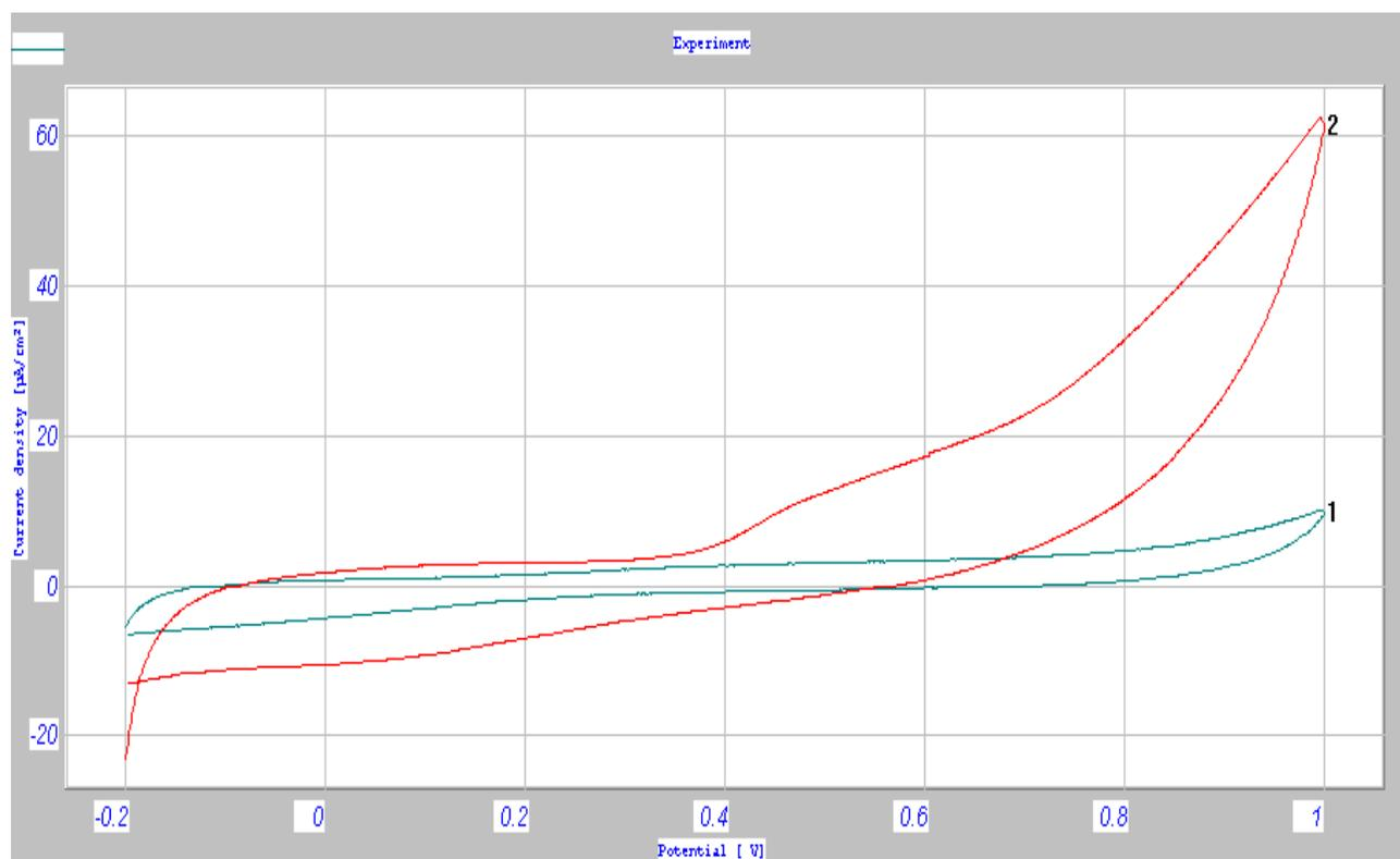
Figure 6. Cyclic voltammograms of *V. opulus* bark at pH=7, 1: 1- electrolyte solution; 2 – *Viburnum* extract.
