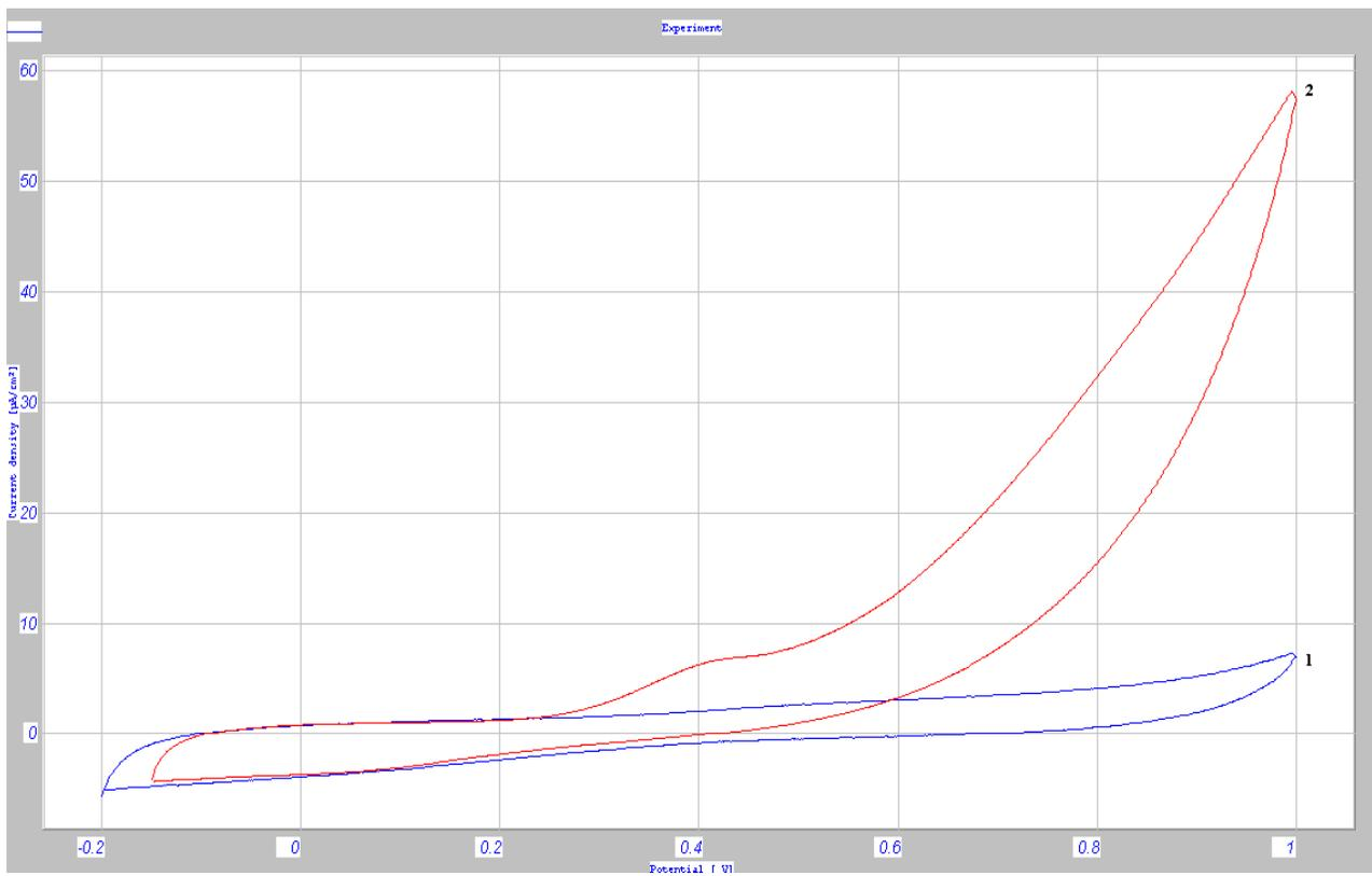
Figure 8. Cyclic voltammograms of *S. ebulus* leaves at pH=7, 1: 1- electrolyte solution; 2 –*Sambucus* extract.
