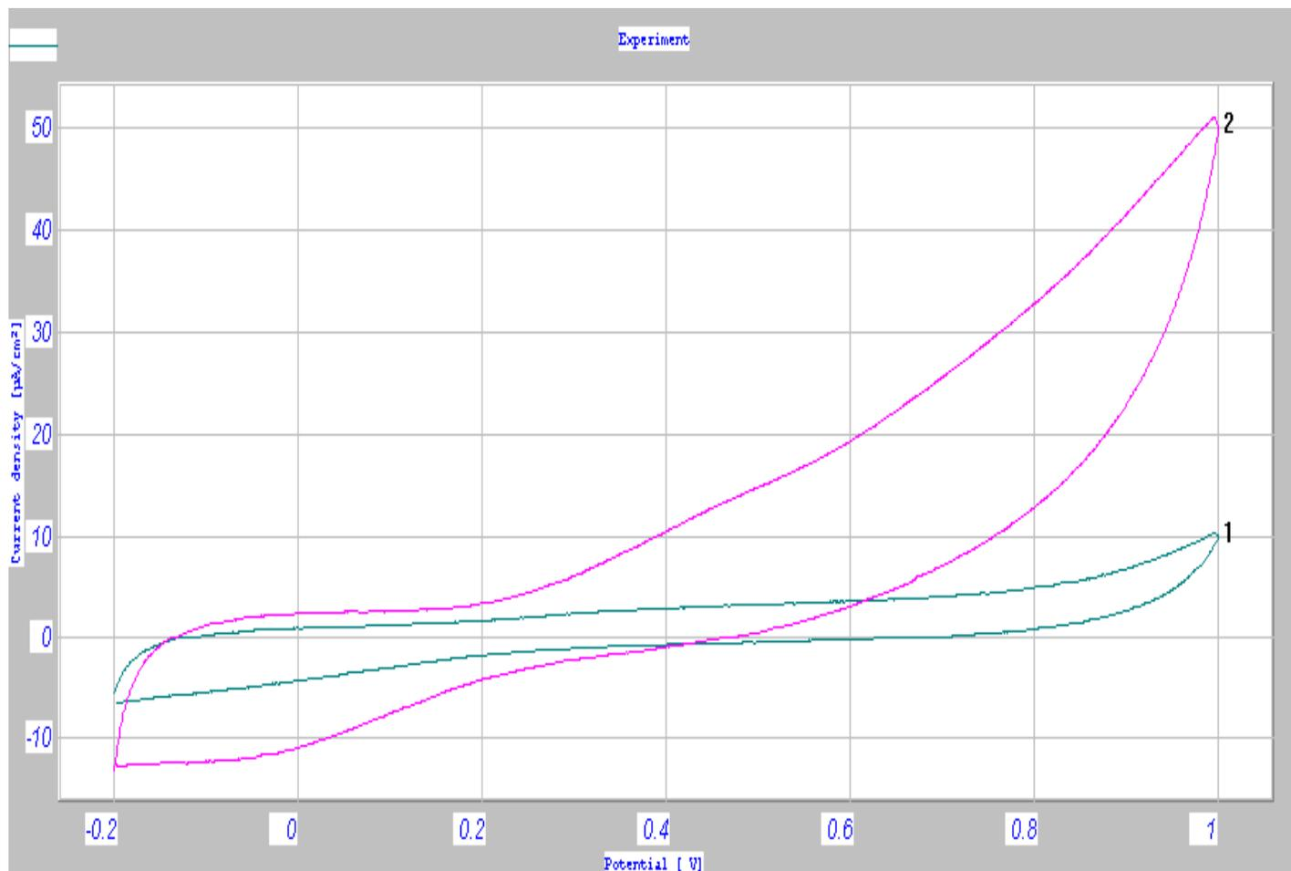
**Figure 9.** Cyclic voltammograms of *S. ebulus* leaves at pH=2,8: 1- electrolyte solution; 2 –*Sambucus* extract.
