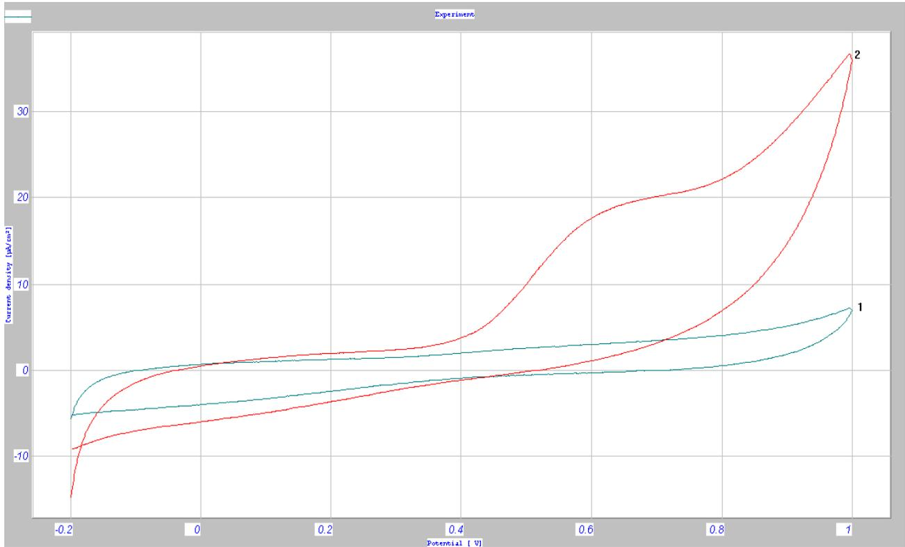
Figure 7. Cyclic voltammograms of *V. opulus* bark at pH=2,8: 1- electrolyte solution; 2 –*Viburnum* extract.
