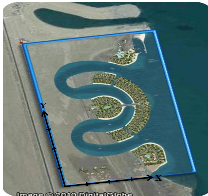
Figure 1b. Domain for simulation as proposed. 1 cm in x - direction = 242 m; 1 cm in Y - direction = 191 m.
