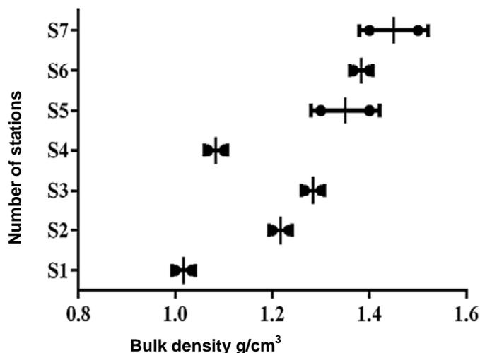
**Figure 2.** Bulk density analyses of collecting marine sediments.
