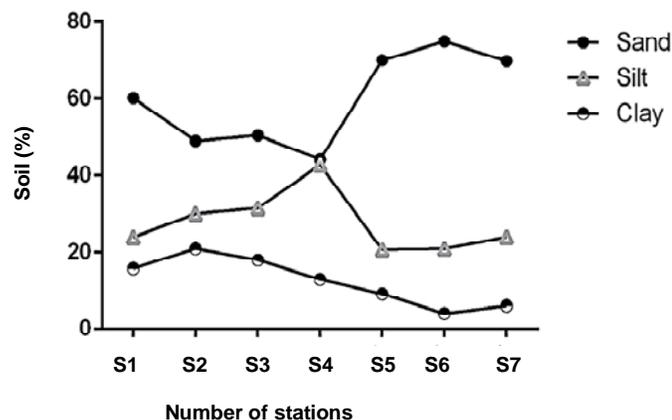
**Figure 3.** Particle size measurement of collecting marine sediments.
