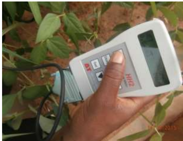
Plate 3. moisture determination using the WET sensor to monitor moisture levels during experiment.
