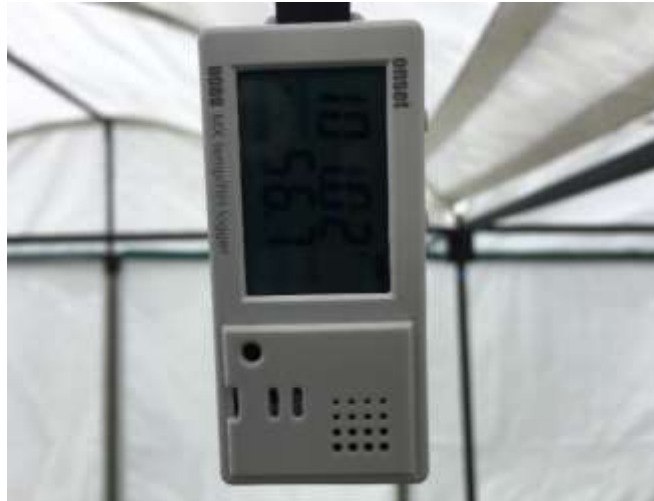
Figure 2. An Onset HOBO data logger inside of a pollen control tent.
