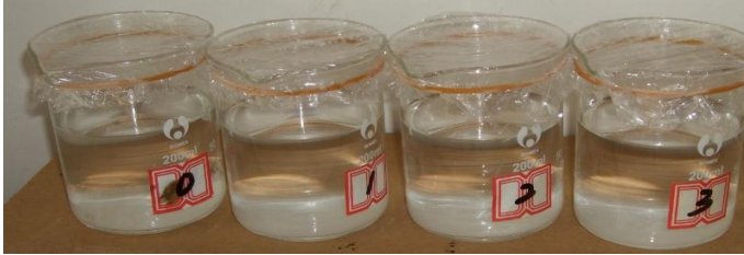
Figure 4. The formation water with dissolved foaming agent on the sixth day.
