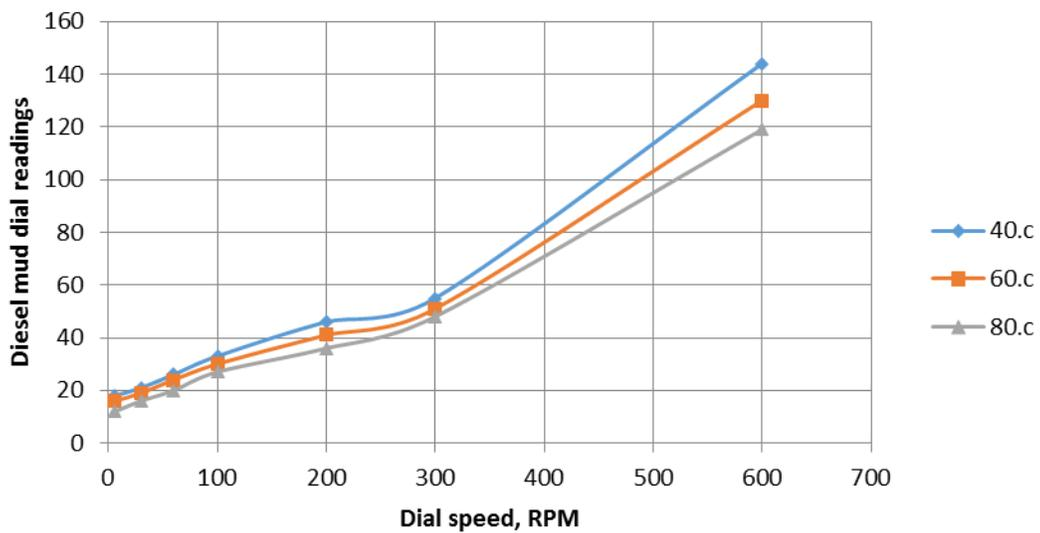
Figure 17. Viscosity of diesel OBM at different temperatures.
