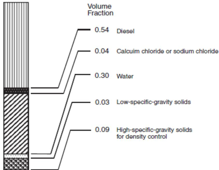
**Figure 1.** Components of an oil based mud.
