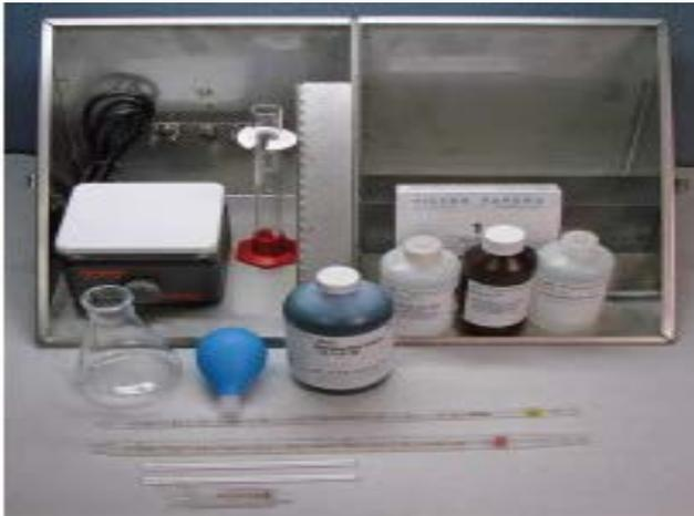
**Figure 9.** Methylene blue kit.
