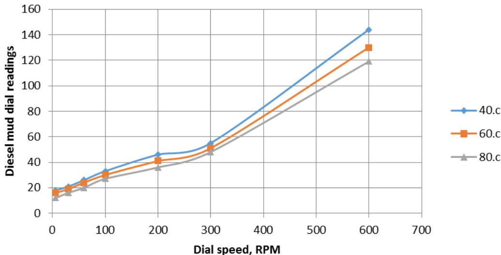
Figure 13. Viscosity of diesel OBM at different temperatures.
