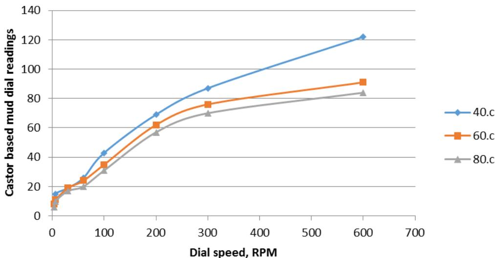
Figure 14. Viscosity of castor oil OBM at different temperatures.
