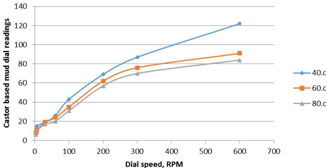
Figure 18. Viscosity of castor oil OBM at different temperatures.
