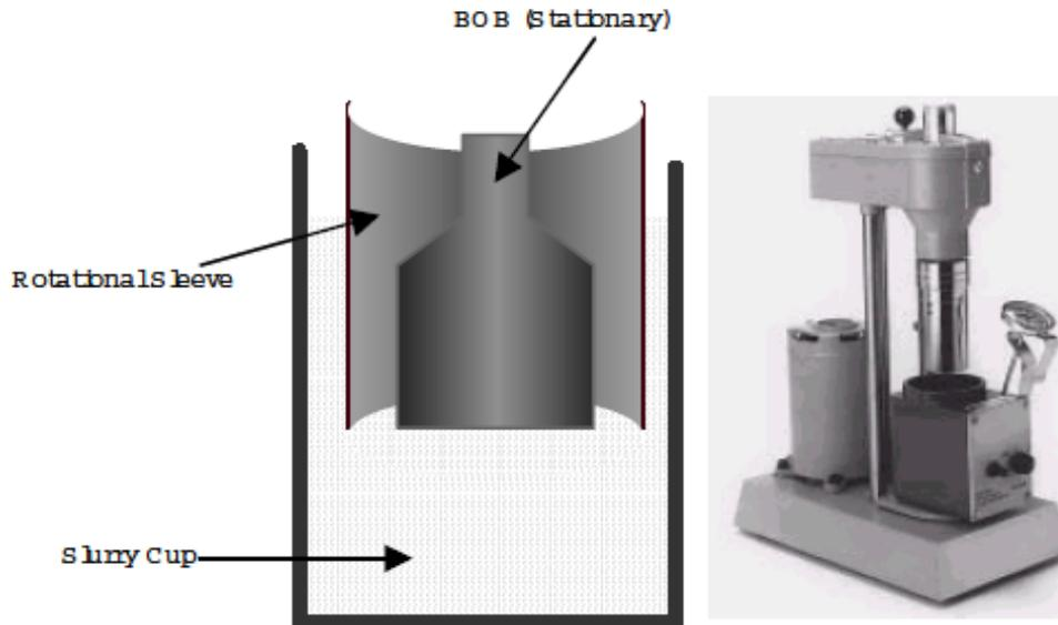
**Figure 7.** Fann Viscometer.
