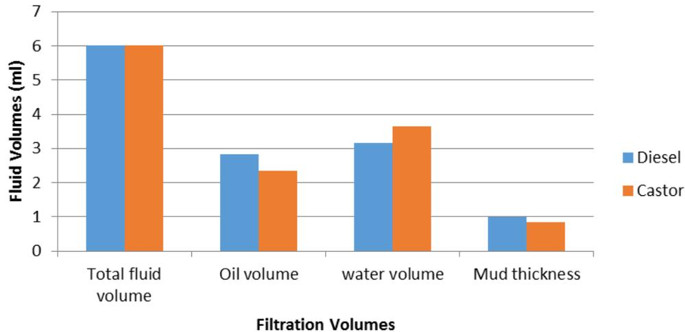
Figure 19. Filtration volumes of castor and diesel mud.
