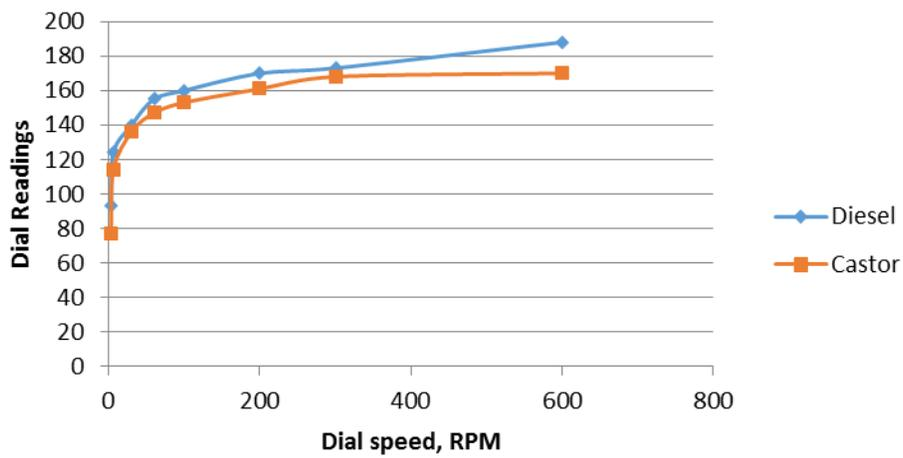
Figure 16. Viscosity readings of diesel and castor oil mud samples.
