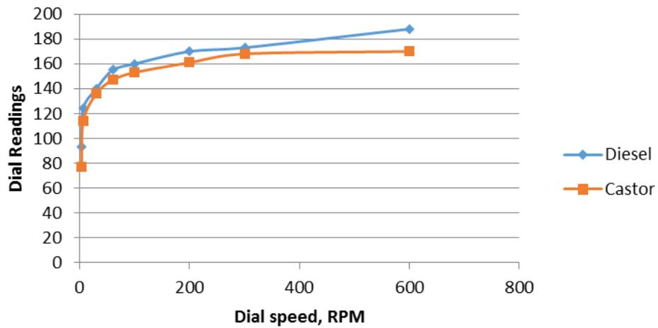
Figure 12. Viscosity readings of diesel and castor oil mud samples.
