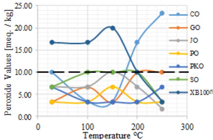
Figure 5. PVs of oil samples with PG additive.
