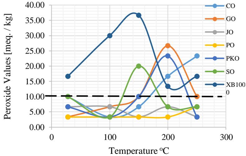
Figure 3. PVs of oil samples without additives.
