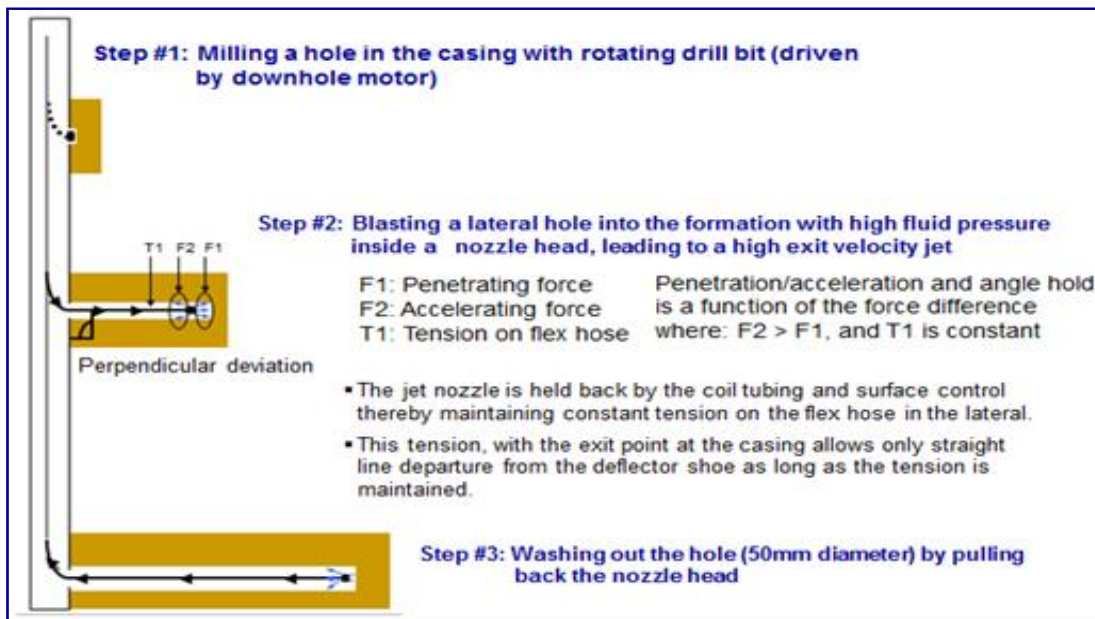
Figure 2. The three steps for radial drilling process.
