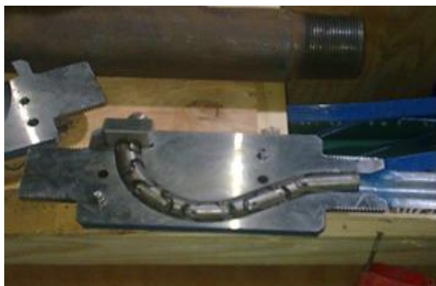
Figure 3. Deflector shoe with flexible shaft inside.
