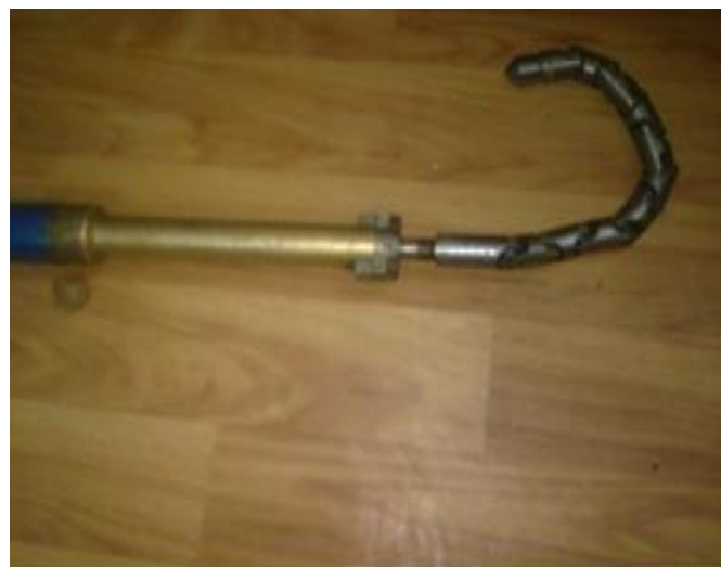
Figure 5. The 1 3/4" bit and the flexible shaft connected to motor.
