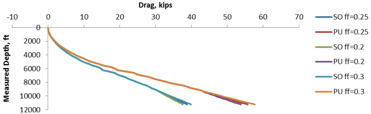
**Figure 5.** Drag plot for case 1.
