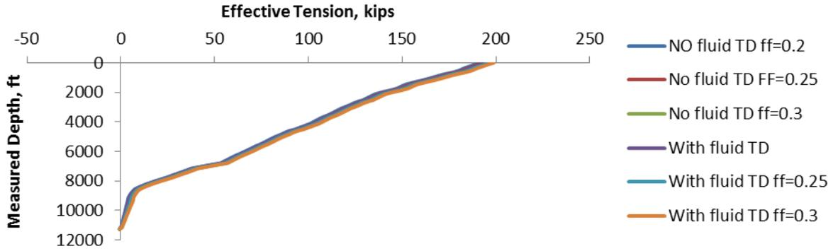
**Figure 9.** Tripping out effective tension plot for simulation with and without viscous fluid effects.
