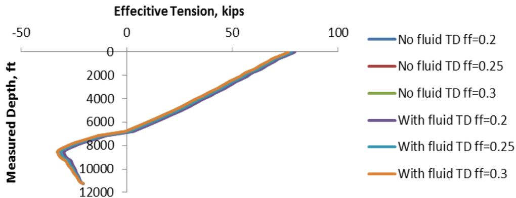
**Figure 11.** Sliding effective tension plot for simulation with and without viscous fluid effects.
