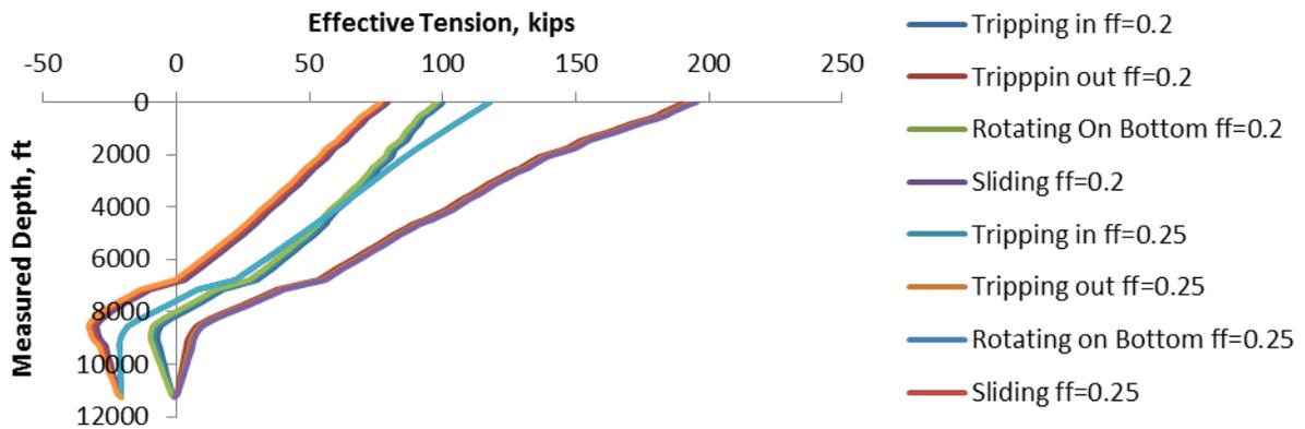
**Figure 3.** Effective tension plot for case 1 (without viscous fluid effect).
