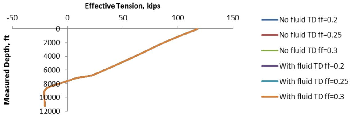
**Figure 10.** Drilling effective tension plot for simulation with and without viscous fluid effects.
