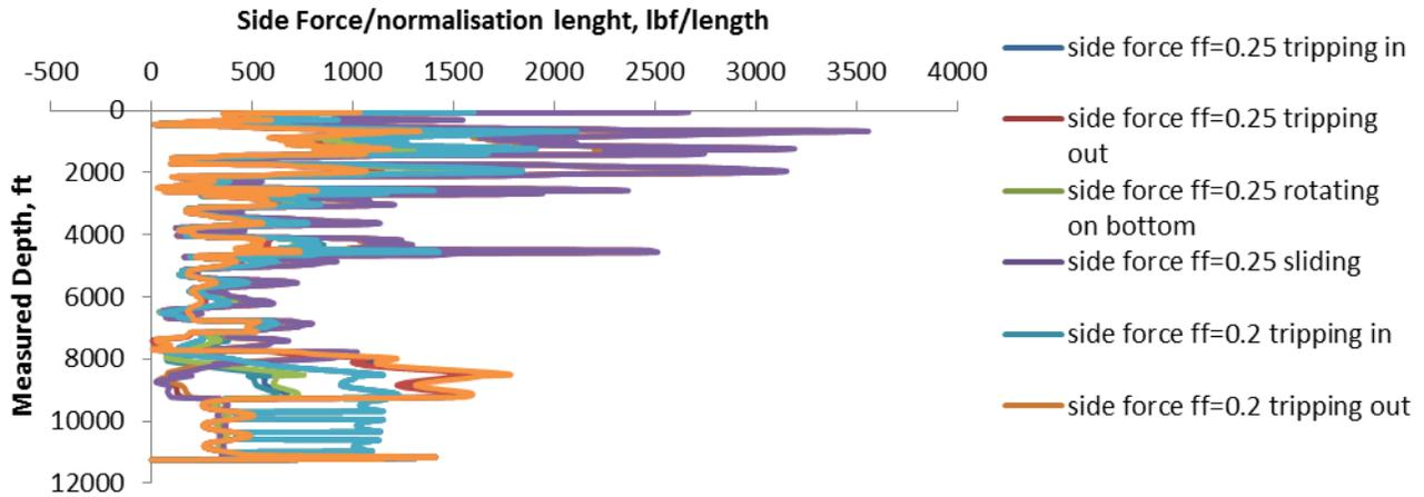
**Figure 7.** Side force/normalization length for case 1.
