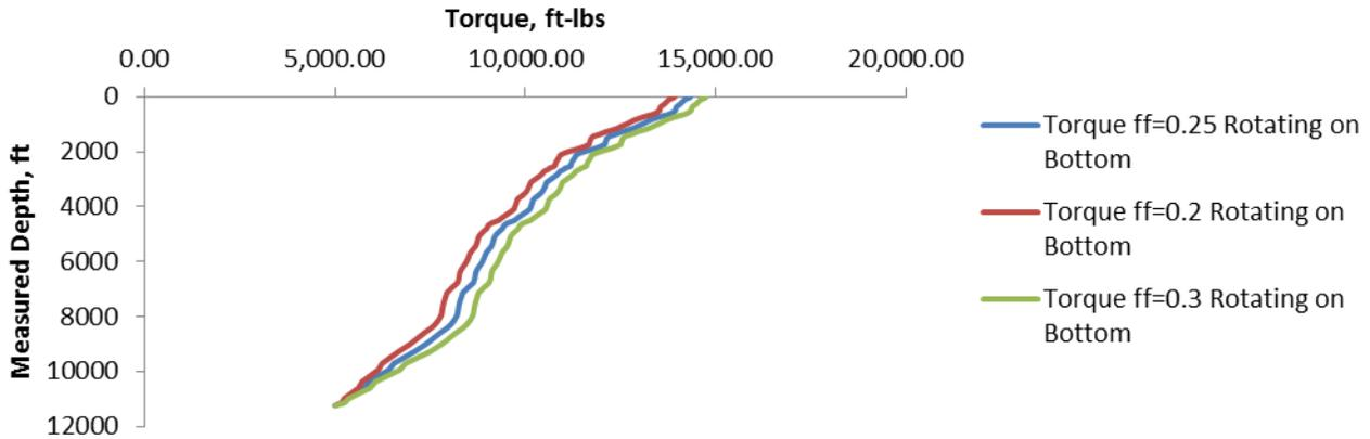
**Figure 6.** Drilling torque plot with no viscous fluid effects. Source - Plot generated by Well plan software
