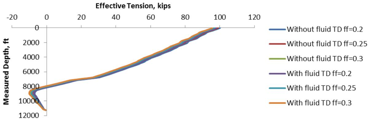
**Figure 8.** Tripping in effective tension plot for simulation with and without viscous fluid effects.
