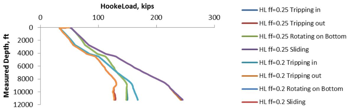
**Figure 4.** Hookeloads plot for case 1.
