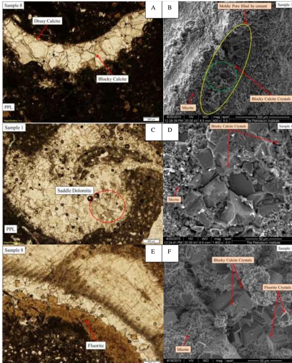
**Figure 5.** (A) Blocky calcite fully filled the pores, (B) Enlarged view of the blocky calcite cement filling the pore, (C) Saddle dolomite, (D) blocky and drusy calcite cement filling the pores with micrite, (E) Fluorite (light orange-brown color) filling the pore, (F) The cubic fluoride crystals along with the calcite crystals (Bera and Belhaj, 2016).
