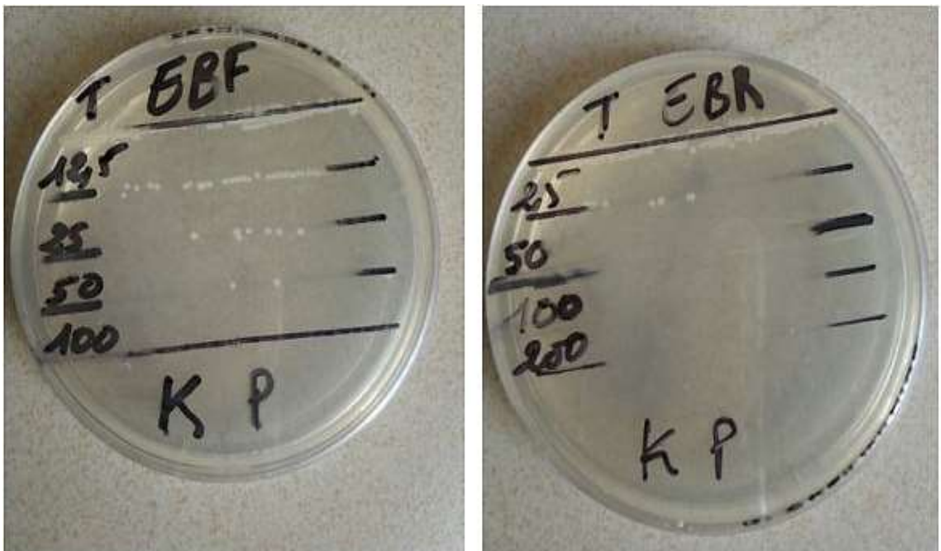
Figure 5. Determination of the MIC of Klebsiella pneumoniae . Kp = Klebsiella pneumoniae ; T = Control; EBF = Leaf ethanolic extract; EBR = Root ethanolic extract; 12.5, 25, 50, 100, 200 represent dilutions of extract (mg/mL).
